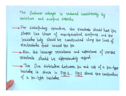
So, therefore the flash over voltage is reduced considerably by moisture and surface deposit for satisfactory operation the rain sheds should have the shapes like those of equipotential surfaces and the insulator bodies should be constructed along the lines of electrostatic field around the pin. I will come to that around the pin means pin insulator
