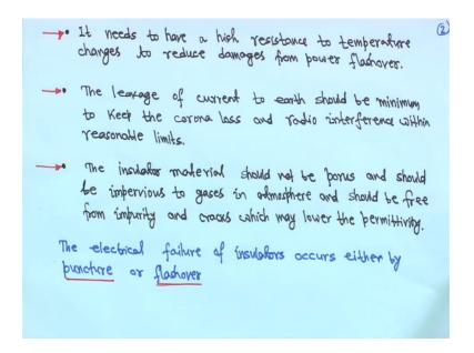
So, it has to have this thing your high your resistance to temperature changes to reduce damages from power flash over. This flash over is very common right and second thing is the leakage of current to earth should be minimum to keep the corona loss and radio interference within a reasonable limit this corona loss thing will come later you have a we will discuss corona loss also but later, so that will come after 3 or 4 chapters.
