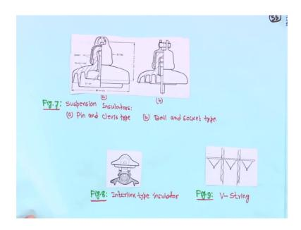
Then, so basically a galvanized cast iron or forged steel cap and a galvanized forged steel pin are connected to the porcelain the cap and pin type your construction, so the units are joined together either by a ball and socket or clevis pin connection this is that (Refer Time: 28:18) or suspension pin insulator this is a pin and clevis type, this is your the same as cement this is porcelain cell right this is the cap and this is ball and your socket type right.
