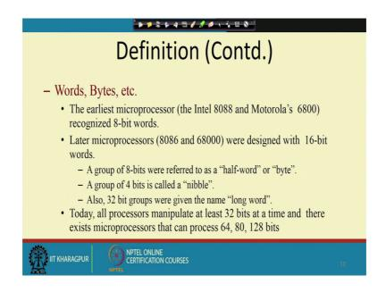
So, words bytes etcetera. So, that the earliest microprocessors they recognized 8 bit words, so 8085, 8088 and this Motorola 6800, 6800, they are all they handle 8 bit words. So, processors like 8086 and 68000 they were designed as 16 bit word.
