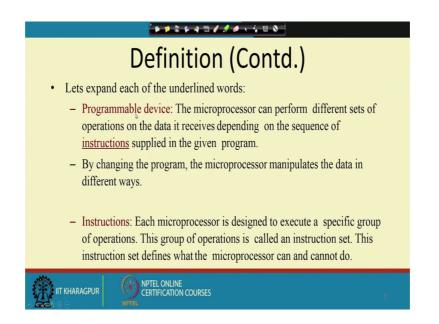
So, first term that we have is a programmable device. So, this is the best thing. Like if I am asked to design some circuits I can design the circuit which will do that operation only. For example, if I am asked to design a circuit that will that will scan one input bit stream and whenever it finds the pattern 4 ones followed by a 0. So, it will output a 1 otherwise the output bit is 0.
