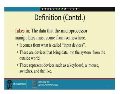
So, next part is that takes in. So, what is the value that it takes in? So, I said that it does some manipulation on the data that it takes. So, it can come from the input devices. Like I can have a number of peripheral devices connected to the microprocessor. So, we have seen that any processor can be connected to the memory as well as it can be connected to the IO devices.
