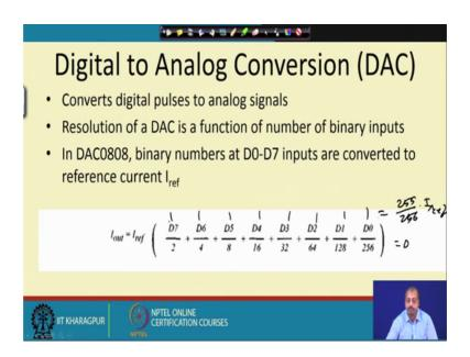
So, so far whatever we had seen this analog to digital converter. So, they are useful for doing this conversion of analog data to digital. So, that is basically acting as the input part of the input part of the interface, sometimes we want to control some output device for example, if there is a fan that is rotating and you want to control the speed of fan. So, digitally if you want to do this.
