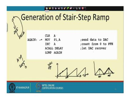
Like if you want to generate some stair step type of ramp then what we do see the we want to generate. So, let us trace this program. So, initially the we have got clear if A equal to 0, initially A equal to 0 and then MOV P 1 comma A. So, MOV P 1 comma a so this statement will be putting this a output on to this a a output will be put on to this input to the 0808. So, it will be converting into a digital value. So, you will get a 0 at the output.
