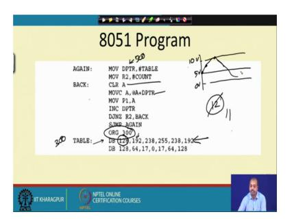
So, assume that this table is the stored from address 300. So, this table is stored from address 300 here and then am storing all the value 128 192. So, so it is 0 to all 30 degree then all those angles. So, that way it is stored and then for each of them I have to output the corresponding wave. So, what do I do?
