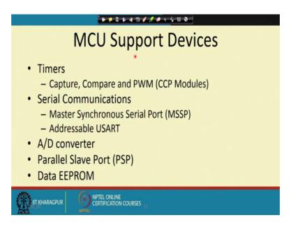
So, there are a number of devices that are supported by this processor like this a timer so, it will capture compare and this pulse with modulation so, this will be all this can be done by this timer. Then there are serial communication so, that a done by this Master Synchronous Serial Port MSSP and also have one user.
