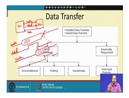
So, if you talk about the data transfer so, there can be parallel data transfer or serial data transfer. So, both these data transfer technique so, you to you can you can divide it into 2 categories, one category is the transfer is initiated by the microprocessor unit or the transfer is initiated by the external device.
