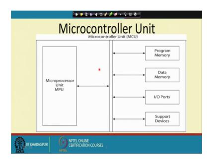
So, pictorially we can see it like this the as if we have got the microprocessor unit or MPU and there are address and data buses. So, the bus so, they are so, this program memory, data memory, I/O port and support devices they are all hanging from the bus ok. So, this is the program and their address and data buses will be there from which the from the MC MPU they are connected.
