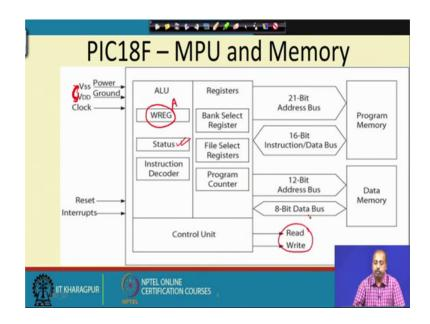
Going into more detail so, this MPU you can divide it into 2 major portion, one part is the ALU part where it will be doing the arithmetic logic operation and the other part is the register part so, it will be doing the register operation. So, this PIC18F family so, it has got 21 bit address bus that is 2MB of memory program memory and 16 bit instruction or data bus.
