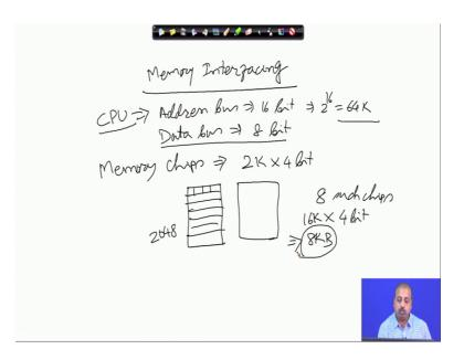
So, this is done by the by the set of topic which is known as the memory interfacing problem. So, we will start with an example suppose I have got a processor to the CPU where the address bus is 16 bit. So, it can go for 2 power 16 locations that is 64 k locations, and the data bus the data bus from the processor it happens to be 8 bit fine the data bus is 8 bit that is once the processor accesses a location. So, it is expecting 8 bit of data from there.
