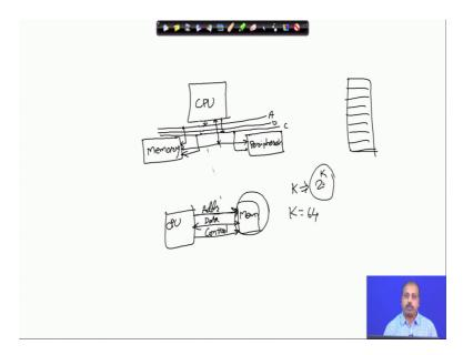
So, in any computer system, so you can find some components like this the basic component that we have, one is the central processing unit or the CPU and we have got two major components which are apart from the CPU, one is the memory one component is the memory and the other component that we have are the peripherals the peripherals.
