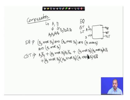
Now so we can have this combinational circuit so it can be used for realizing various module like, we can you realize something called the comparator you can realize something called a comparator, so in a comparator what happens is that the basic comparator module so if I want to compare between the numbers a and b where A and B so both are 4 bit number so this is say A 3, A 2, A 1, A 0 and this is B is B 3, B 2, B 1, B 0.
