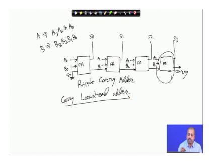
Now, so this way I can add two 1 bit number with the carry also now if you want to add numbers that are that has got the that have got more number of bits like say suppose I want to have say two numbers A and B where is say 4 bit so A 3, A 2, A 1, A 0 these are the 4 bits and the number B it has got again 4 bits B 3, B 2, B 1, B 0 and I want to add them.
