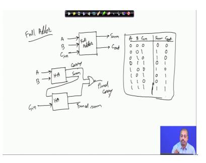
So, the full adder the full adder part so as far as the block is concerned. So, it has got the inputs like this A B there is a third input which we conventionally call carry in to indicate that this is the carry input from the previous stage of the adder and the sum we have got sum output and for this stage we have got the carry which we called carry out that is the carry of the current stage, so this is this is this the full adder.
