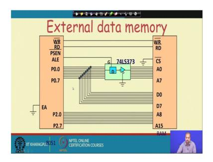
So, for external data memory access, this is the thing that is a right bar line is connected to write bar read bar line is connected to read bar PSEN bar. So, PSEN are is not necessary in this case. So, if the connection is not shown here PSEN bar is not meaningful ALE is ALE signal is connected to G. So, rest of the thing is unaltered. So, P 0 to 7 goes to this latching of latching of this lower order address bus here and the data bus is connected to D0 to D7.
