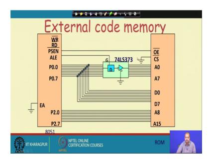
Register. So, this how this connection is done like external code memory so for external code memory connection. So, we have got this um this higher order address bus P2 provided by Port 2. So, 2 point 0 2 to 2.7 they are connected to A to A 15 then Port 0 provides the multiplexed address data bus.
