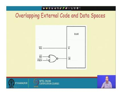
So, next we look into how can we overlap this external code and data spaces. So, this is very simple because if we if like instead of using a separate EPROM for storing the program. So, many cases what happens is that we put with the micro controller our single externally you put a single RAM chip and in that ram chip. So, it acts both as program memory and data memory.
