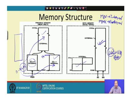
So, if you look into the memory structure that we have. So, the program memory structure is like this. So, we have got this the total address space total address line that 8051 has is 16 bit. So, that is address bus is 16 bit. So, the address total address range is 0000 to FFFF.
