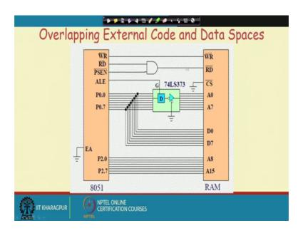
Low this read bar line will be low. So, we will get that corresponding signal here telling that it is a it is read operation similarly write bar line is connected to the write bar pin of the RAM. So, rest of thing we have already discussed. So, this is the only additional thing that we have to do this putting off and of read bar and PSEN bar for doing the overlapping of code and data spaces.
