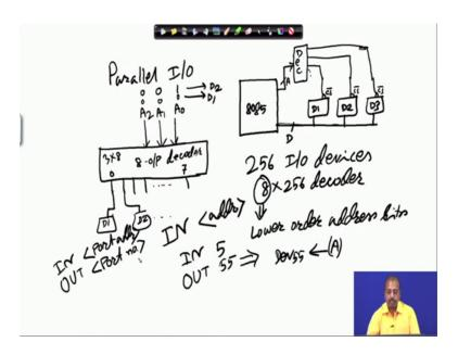
So, this is, basically comes under the broad heading of this parallel IO operation parallel input output operation. So, as we said that in my processor if this is the 8085 processor, then I can have a number of devices connected can have a number of devices connected. So, they are not memories, they are different IO devices D1, D2, D3, like that.
