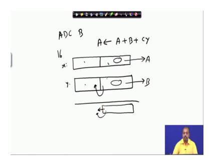
So, the instruction is like this. So, ADC B, what it will do? The register A it will get the content of A plus B plus the carry flag. So, many times it is necessary like if you are doing a multi byte addition like say if you are, you know that 8085 bit allows you to do only single byte addition, but if I have got numbers that can be represented in 16 bits. So, what we do this 16 bit number is consisting of 2 8 bits. So, this is the first 8 bit this is the second 8 bit.
