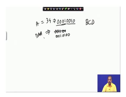
So, for example, if the number is say 34, in the binary number system, this will be stored as 10010 and these bits are 0. So, this is the 8 bit pattern; this is the first 4 bit and this is the next 4 bit for the decimal number 34.
