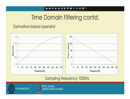
So, here we show the magnitude response here and the corresponding phase response is also shown here. So, from that we can get, it is a high frequency filter and having a linear phase. So, we stop here for the session.
