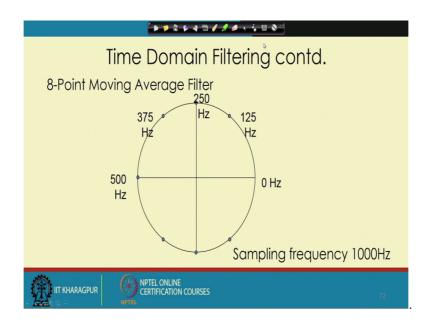
So, here first look at the pole 0 diagram. What we get, the zeros are located like this at different frequency; that means, that we have, if there is a component of signal at 125 hertz, that will come down to actually 0. If there is a component at 250 hertz that will come down to 0, 375 hertz also will come down to 0, so it is coming in that way.
