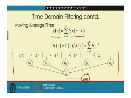
So, the next, in the time domain filtering, we take the technique called moving averaging filters. Now, moving averaging filter actually, helps to get rid of the problems we faced with the synchronous averaging. In case of moving averaging filter, it takes care of the fact that it can work with the single input of the signal. It does not need multiple realizations and thereby it is much more suited for real time operation.
