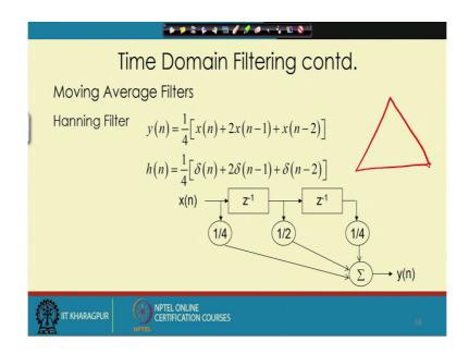
So, now, here we take an example of the moving average filter. Here, in particularly we have taken a Hanning filter. Hanning filter is nothing, but a simple triangular filter. The weights are like a triangle. So, this is a base is a time and we get a triangle and in these particular case that the filter weights what is chosen we have chosen them as integers. So, we can also call these filters as an integer filter.
