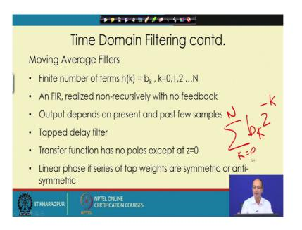
And the transfer function what we got transfer function in these case we got in the form of summation of b K's Z to the power minus K; K equal to 0 to N, that is what the transfer function you got.
