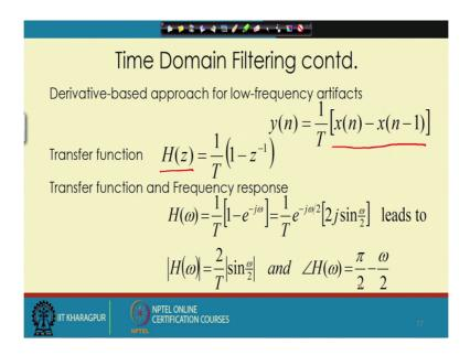
Derivative-based then we can look at the other kind of signals like we can look at that the low frequency artifacts; for example, we have seen that the baseline filter that baseline wandering. So, for the filters what we have seen that is moving average filter, synchronous averaging they are primarily used or good for removing the high frequency noise.
