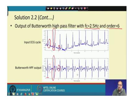
Now, we try further again we increase the cut off frequency to 2.5 for the model order of the Butterworth filter equal to 6 for that again what we see that there is good amount of the distortion in the output waveform the qrs complex is distorted the t wave is distorted here in the output.
