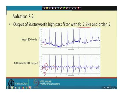
Now, let us move forward we move the that cut off frequency further away from 0 it move to 2.5, we see that the oscillation has moved in such a way it looks like the t wave is almost inverted and the difference between the that q and s point, it has increased with respect to the input signal. So, distortion is much more in this case and for our p wave also I think some amount of distortion it is there though it is you cannot put into words that amount of distortion.
