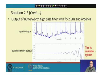
Waveform is completely lost increasing the frequency further to 2.5 cut off frequency moving to 2.5 helps to make the situation better, but the signal initially it is about 0 then it is we can get that it is building up. So, again it is a very unstable filter ok, it is again
