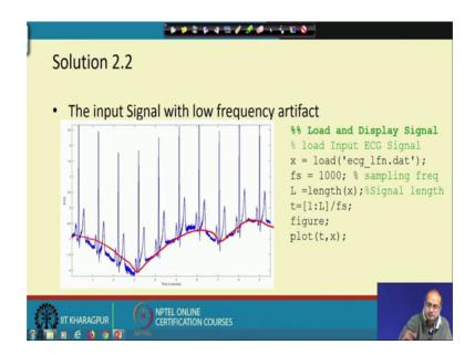
And now let us proceed; just look at the signal at the low frequency noise. So, for that first, what we do? We use the command load to load the signal, we store it in the variable x, then we initialise the variable fs with the sampling frequency 1000, then we find out
