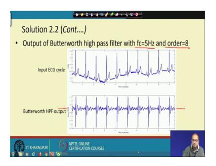
So, let us look for the another case that if you go for cut off frequency 5 hertz and model order 8, we could get again a stable filter and it is successful in removing the that baseline artifact, but what we see the signal distortion is too high. So, again because of the signal distortion due to the loss of the input signal energy between 0 to 5 hertz that this filter makes it unusable for the baseline artifact removal.
