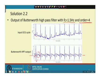
So, now let us again try to increase the cut off frequency again and from 0.5, it is move to 1.5 and model order kept constant as four again what we notice, though it is successful in removing the baseline and keeping it to the value that a horizontal line passing through 0 the signal distortion has again come back the t wave it looks like flipped the difference between the q and the s wave that has increased compared to the original signal.
