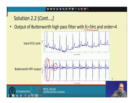
Next, we look that another attempt by increasing the cut off frequency we see the distortion have increased and overall qrs complex, it looks entirely different not only that the p wave is destroyed the t wave is destroyed. So, the overall signal, it looks completely different in this case ok. So, this is also not a desirable filter for our application.
