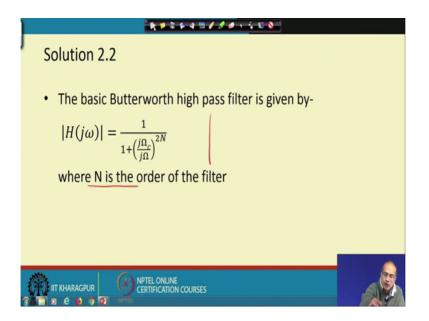
So, now let us look at the structure of the Butterworth filter which is given here and this is the expression of the Butterworth filter for the order n ok. So, we need to make use of that to create the high pass filter Butterworth filter and we need to see that what is the impact of it on the that signal.
