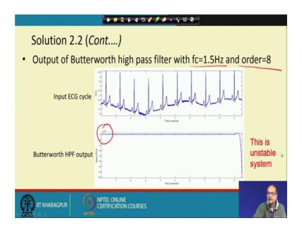
So, these has to be rejected. Next we look at that that again keeping the model order eight we increase the cut off frequency again we see the same problem again we end up with a that a unstable filter and that the transient is going pretty long and we are unable to get any desirable output or rather our signal.
