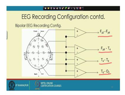
Now, let us look at a one more different configuration, this is bipolar EEG recording configuration. In this case the simple two actually leads are taken positive and negative and as we connect at two points as marked by the 10 20 system, we get the potential or the potential difference of these two points. Like here the first case it is a difference of potential of that F P 2 and F P 8.
