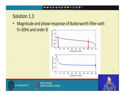
Next, we look at that it more clearly in a bigger way, we see that that magnitude and the phase plot and then we would change the cut off frequency and the order go for the second case where we have the model order is 8 and the cut off frequency is also increase. So, with a increase with a cut off frequency, we see that we can see these constant portion more clearly and it has come up to say 20 hertz is constant up to that after that there is a decrease and the decrease is more pronounced ok.
