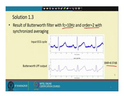
So, first case; we have taken the Butterworth filter with cut off frequency 10 hertz and
