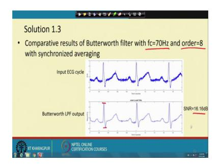
Next, we move for cut off frequency as 70 ok, a big jump model order remains the same as 8, in this case, what we find that there is not much change in the that signal height though, it may look a little better and where we more closer to the qs complex is close to the original signal, but a low not of noise is keeping in, but still it is better than probably that cut off frequency equal to 20 and the SNR also tells as the same thing ok.
