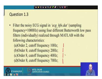
Second is we have model order increase to 8 and that the cut off frequency is also increased to 20, then keeping the model order same cut off frequency increased to 40, then 70 ok. So, cut off frequency is increase means in a low pass filter that we are allowing more and more high frequency part. So, we have to see that how it helps to preserve the signal component that is ECG signal in hand and how it is successful in blocking the high frequency noise ok. So, that is the task at hand.
