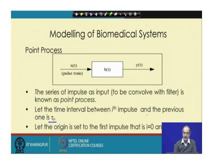
In this case we get the input that is given by a train of impulses and, we have a transfer function which gives rise to our signal of interest that is represented as y t. So, when there is a train of impulse, which is convolved with a filter that is called a point process. And in this case that what is very important is the that inter pulse interval the time interval of the i-th pulse with respect to the previous pulse and we represent that here as t i.
