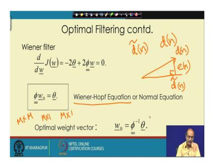
That by substituting those values of that derivative of those 4 terms, we get for the wiener filter that. We get the first time that derivative of the standard deviation of the desired signal contribute to 0. And for the second and third term that is contributing minus 2 theta. And the 4th term is contributing this part that 2 5 w.
