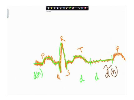
The ECG signal is having that P Q R S and T waves. This is P Q R S T and because of different kind of noises say high frequency noise, then we have that power hump. Actually, lot of noises are added with it and it got smeared in this way.
