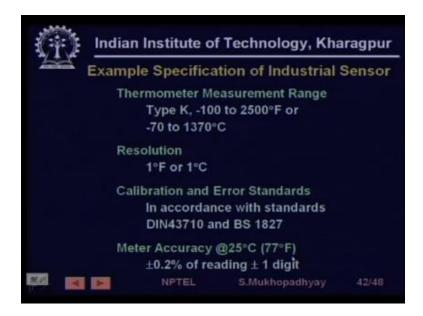
So similarly it says that the that the meter accuracy at 25 degree centigrade hat is when the ambient temperature is 25 degree centigrade is 0.2% of reading  $\pm$  one digit this  $\pm$  one digit comes because you are going to have a digital display, so we see that in digital displays there has to be a there is a there is an effect called quantization.
