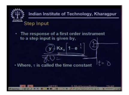
So if you have a step input so the first kind of input that we consider is a step input so step input means it is it is at zero and then suddenly it rises so t=0 the input is 1 suppose so then we actually we can you can compute that the time response or y(t) is going to be such a function of time, so the graph will show what kind of function it is.
