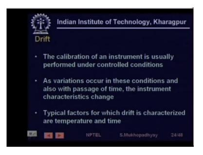
So typically drift is characterized for temperature and time.
