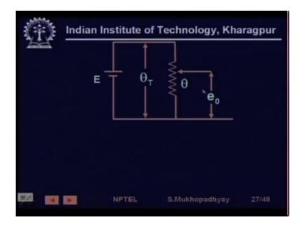
So this potentiometer will be connected to this variable points as the variable point moves the voltage that you will get will be directly proportional to the to the position right, so in this case there will be instant to instant and since the position is the position is actually a mechanical variable so therefore there is not going to be too fast movement, so as far as so the electrical behavior is so fast compared to that.
