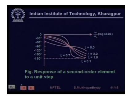
So you have similarly the phase if you see the phase the phase plot looks like this again with frequency so towards low frequency the phase is phase tends to stay small and as freaked as frequency increases so this maximum phase that can occur is for is 180 degree, so these are the phase lags.
