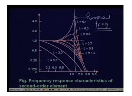
And this is the expression for this is the plot for gain so you see that the gain actually changes with frequency right and for under damped systems the system tends to be tends to resonate so this is the resonant frequency so if you give a sinusoid close to the resonant frequency then you get a huge output right on the other hand for over damped system there is there is there is no such resonance. (Refer Slide Time: 13:12)
