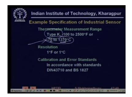
So this is for example an industrial thermometer, so see what it says what all are stated so first of all it is it is based on a thermocouple therefore the type of the thermocouple is stated we will see what the type of thermocouple is but interestingly the range is given so you see this is that the minimum and the maximum values in which this thermometer can be used with these given specifications.
