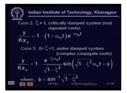
We will just see the case and then we will see the plots so and then we have a case when  $\xi = 1$ ,  $\xi = 1$  which is called the critically damped case here we and the last case is when we have  $\xi$  is less than between 1 and 0, so that is called the under damped case.
