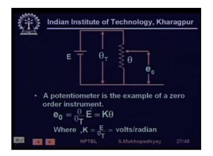
So the output voltage will be directly proportional to the displacement  $\theta$ , let us say angular displacement in this case if potentiometers can be angular as well as linear.
