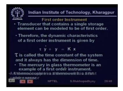
So if so we can easily compute the response of us of a sensor whose input is a step input so we can so let us try to characterize the response of this kind of a sensor to various kinds of changing inputs so the first so these are two examples marketing glass thermometer and thermocouple thermo well.
