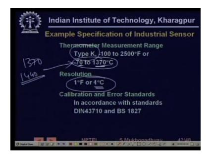
So it is so the minimum change that can be observed change which can be detected by the sensor is actually one degree centigrade.
