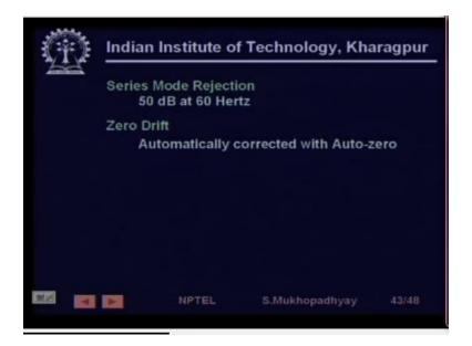
Now since thermocouples use long wires so there is a series mode rejection since mode rejection means that typically with thermocouples are drawn from long wires so they typically tend to catch series mode interference especially at the power frequency so because there may be power lines and they will they will add power frequency interference as a series voltage.
