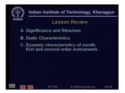
So this brings us to the end of the lesson so what we have done in this lesson is, that we have seen why sensors are so important we have also seen there they general structure we have looked at the static characteristic main static characteristic parameters and like your sensitivity, linearity, accuracy, resolution, spam etc. (Refer Slide Time: 21:03)
