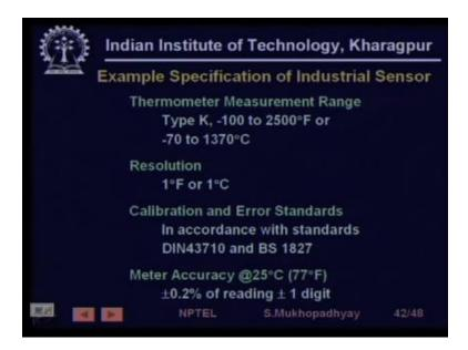
And therefore this  $\pm$  one digit error comes, so basic accuracy is 0.2% of reading in this case it is stated as interms of reading.
