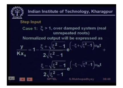
So again it is response to the step input in this case we have three kinds of cases depending on what is the damping factor so one case is when the damping that is zeta is greater than one in which case we call it an over damped system and this is the expression for the output time function.
