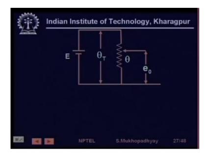
They are a potentiometer when I was talking about a resistance right, so a potentiometer is nothing but a resistance so for a potentiometer the position signals potentiometers typically measure position which.
