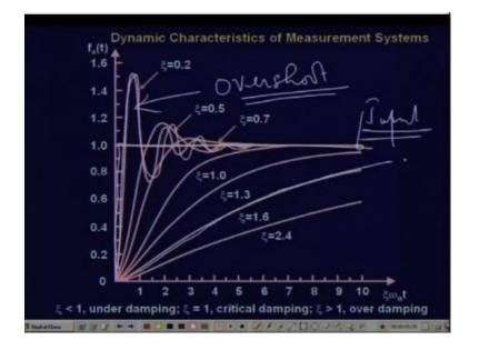
So the plot actually looks like this so this is of interest to us so you see that this is the step response so the you so the input applied is this, this is the input now for different values of Zeta for example if as Zeta goes to lower and lower values you can see that you get an oscillatory behavior so there is an overshoot this is called an overshoot, so for under damped sensors you are going to get an overshoot.
