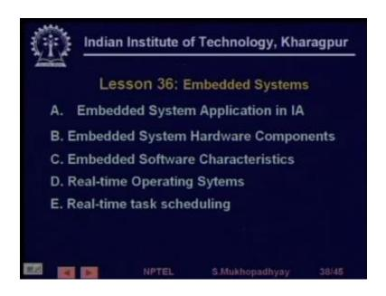
So we took a look at you know embedded system embedded systems and understood is basic hard types of hardware components and basic software characteristic the kind of software that are used in that, then we took a look at you know many of these systems are actually operate for example, a CNC machine, a CNC machine has various at least 3, 4 processor it has axis controllers it has PLCS it may also have you know front-end processors which manage the man-machine interface.
