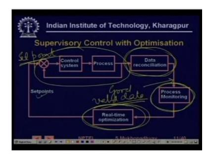
You get an idea as to whether your process is working fine or whether it needs a new set of new set points that is another cycle of real-time optimization will have to be done to generate new set points. So this typically the way in which the Supervisory system is always looking at the plant and then being and carrying out optimizations based on set points.
