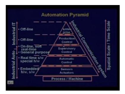
So we first take a look at the automation pyramid remember we had taken a look at this automation pyramid in the very early parts of the course, so here as we said that this is the automation is organic it can be viewed as a pyramid with the process machine with basic equipment the which is the ground and then you have the sensors and actuators which take information and provide control inputs. Then you have the first layer of controls automatic controls and in this course.
