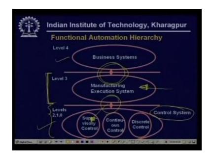
Now given I mean handed down to the Supervisory control system then the Supervisory control system can act according to that schedule and actually do commit execute the steps that are required to do the physical manufacturing, right.
