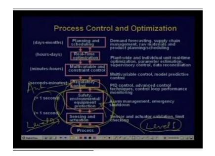
So this is a picture which shows that you know in a typically in a process control situation not an order not a discrete manufacturing scenario the kinds of technologies that are used so you have and also the time scales that I was talking about so you have at the bottom level you have these sensing actuation, protection, alarm systems which typically work at sub 1 seconds kind of time scales.
