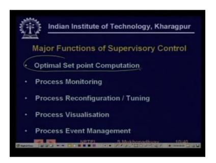
Similarly, one has to do one has to supervisory control always looks at the process and sees with us whether things are going fine for example breakout detection as I was saying that whether by looking at the temperature profile by looking at the mold levels whether it is possible to the system is always monitored such that whether we can detect the possibility of a breakout and then immediately take corrective action, so that breakout does not offer so that would be like process monitoring.
