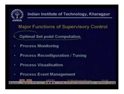
And similarly process event management so you know I mean something keeps some along goes some pressure level suit shoots up one has to find one has to activate strategy is shut down mechanisms emergency mechanisms such that the situation is managed with the least amount of production loss with safety and reliability to the personal and the equipment no so such things are typically handled at level 2 or these are the functions of the Supervisory control. (Refer Slide Time: 22:20)
