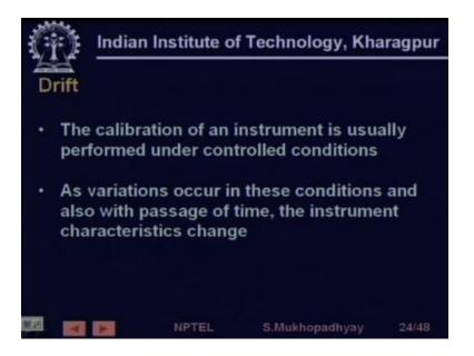
Next is drift so sometimes what happens is that even if you correct even if you correct at any at some point of time during calibration even if you correct for the bias on the gain error you have drifts in the bias on the gain so gain such bias and generals can develop due to you know variations in temperature variations in time or some other conditions so the rate at which it these will develop our are characterized by a performance characteristic or drift.
