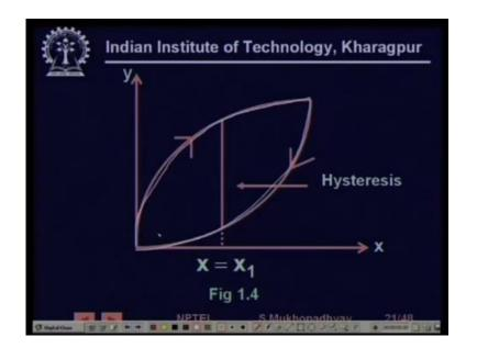
So this is the figure that we are saying that the if X is increasing then the then the readings that we obtain follow this curve while if X is decreasing we actually forward distinctly different curve so if such behavior is demonstrated by an instrument it is called it is said to have hysteresis.
