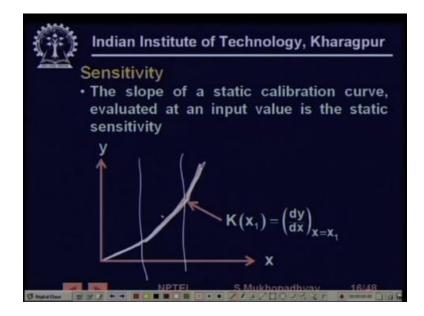
So next we are interested in sensitivity so sensitivity is actually the slope of the line so if you have a calibration curve and then so that that will be the sensitivity and if you have a calibration curve and then get a straight line in case you have a linear characteristic it will have one single sensitivity if it is very nonlinear then sometimes you may also express it as so you can take do actually do various things you can express say let us say three sensitivity figures.
