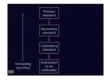
So this is what it says that this is what I was talking about that there are different standards of instruments so the instrument we calibrated can be calibrated against the laboratory standard now the laboratory standard instrument also has to be from time to time calibrated against you know other standards like you know secondary standards which are straight which has special instruments which can be you know existing in some test houses and then.
