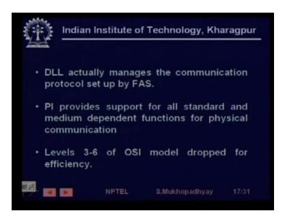
The data link layer actually manages the communication protocol it takes care of the digital communication details error coding parity checking etc... and the physical layer provides a the electrical and medium dependent so if you have wire if you have RF then there has to be radio
