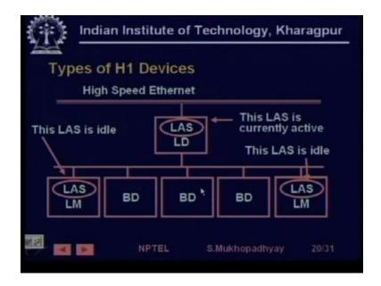
So exactly same diagram this is repeated so these are linked master and their basic devices are not capable of becoming link masters or link active schedulers while link masters are capable of becoming link active schedulers. (Refer Slide Time: 17:07)
