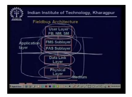
So you have finally the field bus architecture so you have the physical layer the data link layer and the application layer broken up into two parts and then you have the user and user layer which involves feed the function blocks which are you know abstract computing blocks which specify abstract communication let us say between analog input device and a process controller or a process controller and then analog output device.
