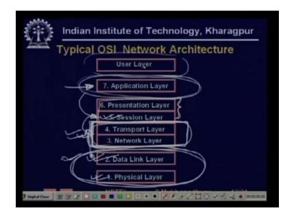
A typical a very generic general-purpose Network these are the general-purpose model and in the various special networks you have a you have some sort of an adaptation of these network architecture in all networks adapt this generic OSI network architecture in certain ways so in the
