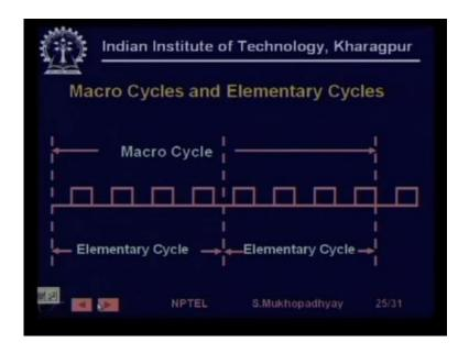
And the communication is actually organized overall into cycles called macro cycles and within each macro cycle so macro cycle is the basic cycle over which the over which the communication is periodic and then within macro cycles you have elementary cycles so an elementary cycle is decided by the fastest by the device which needs to communicate the fastest so you know if you have so let us let us see the next example we will understand it better. (Refer Slide Time: 21:23)
