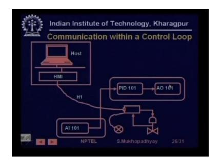
So for example to take this loop this is a PID loop with say an analog input PID and an analog output so these are you actually you know on different devices and the analog input so they are all on the network and the analog input this is a this is a functional block representation so virtually this AI must communicate with PID and then PID by must communicate with AO and they are actually physically different devices.
