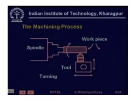
So essentially it is metal removal which means that they actually is removal by a tool which is made of very hard metal things like you know carbide diamond etcetera so essentially we have to you have to produce relative motion against off the job and the tool. (Refer Slide Time: 02:55)
