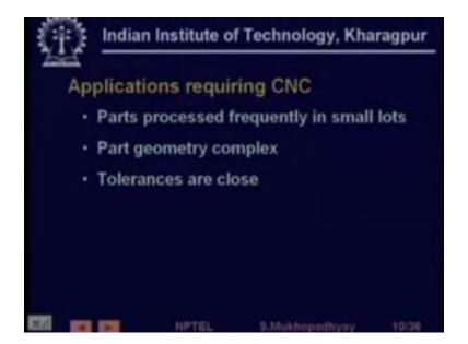
Tolerances are closed because the kind of controls that you apply the kind of controls that you apply are so sophisticated that it is not possible for manual operators to apply such control and therefore very high compliance to the tolerances can be realized.
