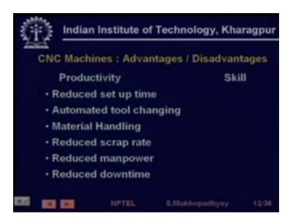
Scrap rate is reduced because you must have it is assumed that the part programs are written with carefully using scientific you know optimization methods so from a given piece of material because you are not going to you have much more precise operation so you can have optimal material utilization therefore scrap rate will be reduced manpower is reduced because much of it much of the work in these machines can done automatically.
