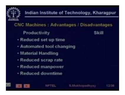
So what all productivity is much improved we do to reduce set of time automated tool changing which is again reduce the set-up time I mean unproductive time sometimes some of these machines will have inherent material handling so if you want to change a tool the machine will stop the machine take out the tool put it in the tool bag as a zing bring out another tool so all these material handling work will be done by the machine itself.
