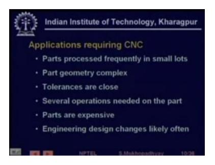
When engineering design changes are again lightly again this is also related to set-up time so you see that there are basically two points one is situations where a good amount of set-up time is required and secondly where situations have situations where very high skills took to cater to complex geometry and close tolerances are required so it is during these for these two reasons that CNCs score over non CNC machines or manually operated machines.
