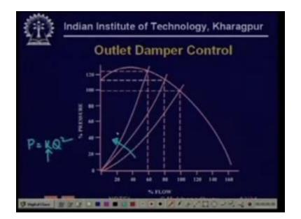
So as the damper is closing this curve is shifting this way because this is increasing k now what is happening to the energy the energy in a fan the energy being delivered is  $P \ge Q$ .
