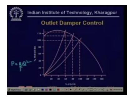
Of  $P = KQ^2$  this K value is gradually increasing which means that as the damper is closing more and more pressure is required to drive a given flow that is natural.
