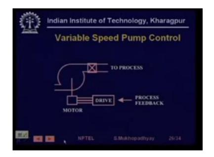
Again for pumps this is a variable speed pump control so you have constant speed drive one way of controlling is either you have a constant speed motor drive and you have a valve or you have a variable speed drive of the pump depending on the feedback depending on the load basically that the drive has to be controlled and some speed references to be given we will see in our future lectures in detail as to how these how the speed of a motor and a pump can be controlled oops.
