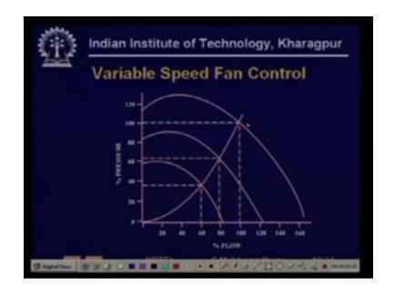
Right so we see this variable speed fan control so now what happens is that if you want to reduce the speed we are not going to put any damper or any valve in other words the characteristic of the system remains unchanged now we are changing the speed of the fan so the fan characteristic shifts. (Refer Slide Time: 12:14)
