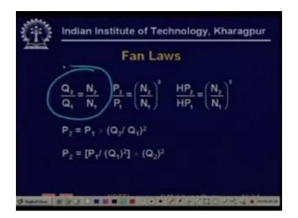
That in a fan roughly Q2 by Q1= N2 by N1 if you operate if you change the speed the curve shifts in such a manner that on the Q axis you are going to get proportional these things and P2 by P1 = N2 by N1<sup>2</sup> square so the horsepower variations.
