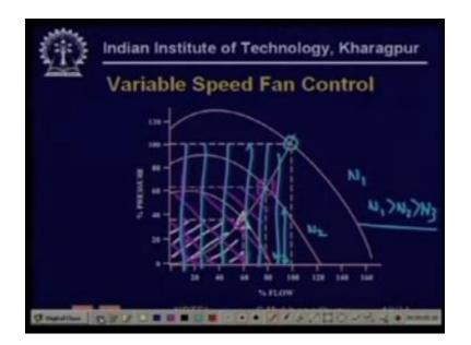
So this is the area required this is the energy and similarly for this case second operating point this is the energy and for the third operating point this is the energy so for the third operating point this is the energy so you can very well understand that energy falls very sharply so that is why.
