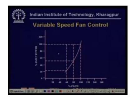
Savings right so you can now see that the power curve how sharply it falls compared to what you had seen in the case of the outlet damper control.
