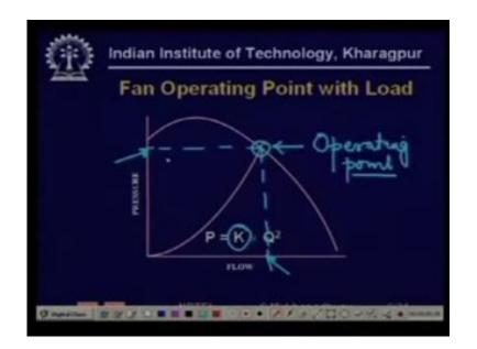
Across the pump then they will they will intersect and this is the operating point, so this is the operating point. So immediately if you if you connect this is the flow and this is the pressure which will be which are going to be established so the pressure which will be established if you connect this pump with this load this flow will be established and this pressure will be established, right.
