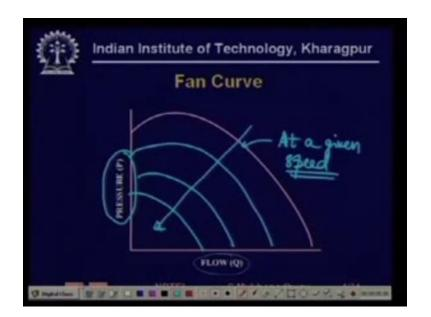
So let us look at a basic characteristic of a fan right, so here we are, the fan is this is the intrinsic characteristic of the fan itself irrespective of what the load is. So the fan actually develops a pressure at it is outlet and also develops a certain flow and this it develops when the fan is rotated at a certain speed so when we have plotted this curve.
