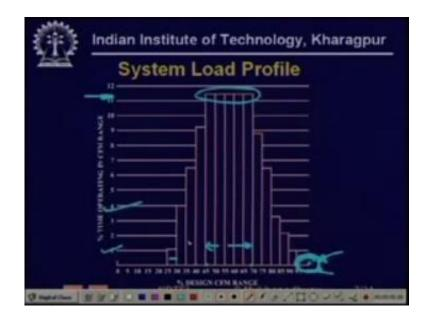
So rather it will operate most of the time at half level and it will also operate at very low levels for a very small amount of time so this is a typical load characteristic. Now let us see what happens so we need to shift this operating point right all the time. (Refer Slide Time: 17:04)
