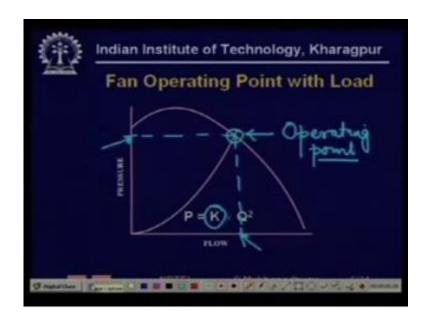
So now let us talk about varying the flow because we need to depending on the load characteristics for example if your electrical energy demand decreases then you need to reduce the rate of combustion. So you need to reduce the flow air flow into the furnace right.
