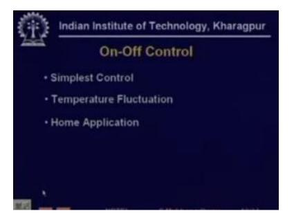
So another very simple method is so out of control is the simplest of control there is step there is going to be temperature fluctuation basically flow fluctuation will cause may cause temperature fluctuation sometimes for home applications it is used when you have less load and you have a large volume so if you so there is a lot of you know you know thermal capacitance so little bit of flow variation will not be felt because of large volumes of room.
