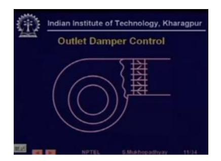
The next control which is used is called the outlet damper control for the fan so outlet damper means basically a damper means you know you see it is like a set of veins you know just like this you know sometimes on the you must have seen what is the word of this call there when you put something on the windows to keep out the sun so you know they are there you can change gaps you can you can move them either you can keep them like this or you can keep them like this so that some air can flow.
