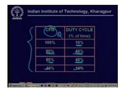
So let us see now what happens if we shift the operating points, so this is summarized so it says that it this is like you know roughly suppose because we are going to see an example so suppose in our example 100% CFM, CFM means again basically flow cubic feet per minute this is CFM means Q so 100% flow stays for 10% of the time 80% flows stays for 40% of the time, 60% for 40% of the time and 40%, 10% of the time. Imagine such a case okay, then.
