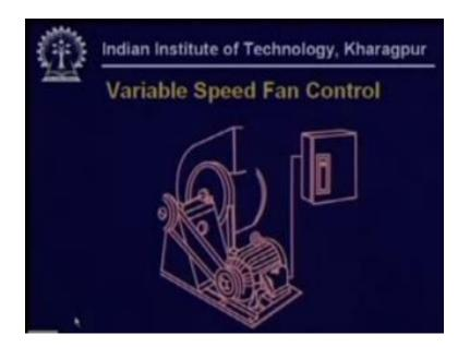
But what is the third method the third method and which is the which is the very energy-saving method is variable speed fan control so you do not put any damper but you rather change the speed of the fan and reduce it when you require less flow but for that you require a variable speed drive of the motor and that is much more sophisticated technology is required especially when the motor is large compared to you know dampers and or valves.
