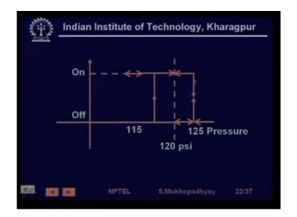
You see what we are trying to do is that if you have we have at a pressure setting they off let us say 100 to 120 psi now as you are drawing load so these this pressure will start falling and then at 115 psi you again turn on the compressor such that the pressure keeps rising and becomes so the pressure will so you actually make the you touch a turn on the compressor at this point of time and then the pressure builds.
