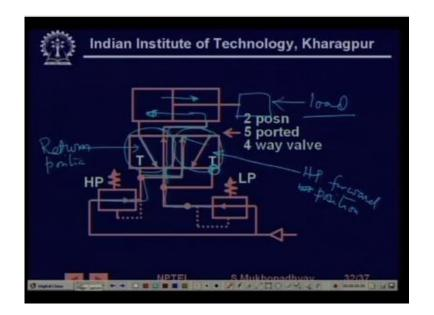
Similarly this is a case where this is at two position five ported four-way valve so five ports because one, two, three, four, five. Five ported and two position because this is one position and this is the other position okay, so what happens is that sometimes you know these Pistons when they are moving the load they will require high pressure operation because a lot of force is to be created and when they are returning then is a low pressure operation.
