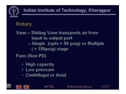
So here also you can have singular multiple stages the other option which is non positive displacement offence they are generally used where high flow volume capacities are needed but at low pressure so in such cases fans are used and they can be centrifugal or they can be axial.
