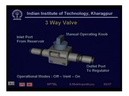
So namely off vent and on so it can be made off in which case air will not flow if it is on then the air will move from inlet to the outlet and if it is in vent mode then the inlet and outlet will be connected to the atmosphere.
