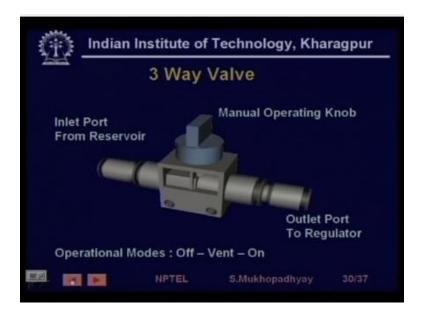
For example at this is a typical three-way valve which is manually operated using this knob.
