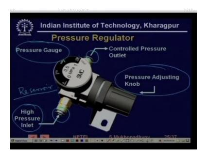
So this is just atypical picture of a pressure regulator and so you have this high pressure inlet you have the low pressure or the controlled pressure outlet so this is going to the system or the equipment where the pressure is needed this is coming typically coming from the reservoir so now the pressure setting can be adjusted by this pressure adjusting knob and often there is a pressure gauge so that you one can see that the inlet pressure variation.
