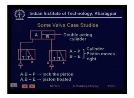
So it can move it is free to move because both ends are connected to vent so yeah so A to AB to P locks the piston and A B to E locks means exhaust the piston is floated.
