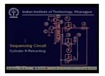
Next last point last point, now cylinder J has retracted fully. So now this pressure cannot so now the pressure here builds up, so the pressure here builds up so the pressure here also builds up and this now pushes the cylinder down but this time no node that it has to pass through this so therefore while the cylinder H is coming down there is there is always a back pressure this is not connected to tank because it is not passing through this it is passing to the relief valve.
