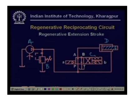
So that is exactly what is being shown here, so you see again identify components first so you have this is say A pump this is B relief valve this is C directional valve and this is D a cylinder, now see that we have drawn the cylinder rod a bit thick just to ensure that the rod area is not negligible to the cylinder piston area this is the piston ad a capital A and this is the rod area small A.
