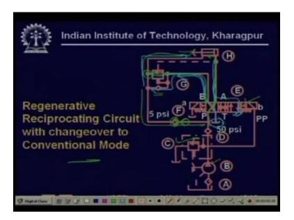
So then what will happen is that the this is this will be the flow, so it will directly flows through this check valve straight and it will comeback directly it will actually come back here and it will get connected to tank so that is a very conventional mode so in this case it will that is there is no pressure requirement and it will it will come back, so on the only advantage is that since we are we have higher force requirement.
