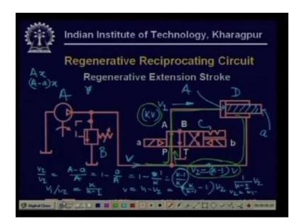
Suppose so what is happening is that now the two side areas are different right also look at this particular directional valve which is to position and it is kind of you know it is depended in the sense that so when you what happens what happens when both the solenoids are off so the both the solenoids are off then it stays in the position corresponding to the last operation of the solenoid.
