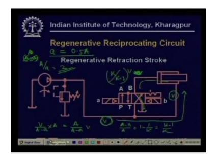
In the retraction stroke in the retraction stroke now you are in this position so now this simply this is the path directly this is the part that is there is no there is no fluid addition or anything so now what is happening is that if this is V then this is V and obviously because the directly goes into this and what is going to be this, this is going to be naturally this will be so a into another (A- a) v.
