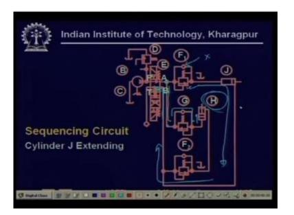
So the moment it comes to a mechanical stop here this pressure will now build up because there cannot be any further flow through this, flow is stopped. So immediately this point rises to pump pressure that will operate this valve, right. Cannot go through this cannot go through this at this point so it goes through this and starts pushing starts pushing valve J so flow goes like this like this like this.
