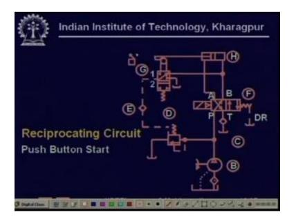
Next what happens how do you start a new cycle so you start a new cycle like this, a new cycle is actually started by pressing a push button, so this coil is has to be connected in such an electrical circuit such that it can be switched off by this limit switch as we have seen at the extent at the end of the extension cycle and it can be switched on by a push-button, so every time you want to start one extension retraction motion you need to switch on this solenoid.
