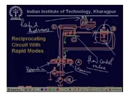
So what we are seeing here you see again let us identify components pump, motor, relief valve this is tank and filter this is a three-position solenoid, electrical solenoid actuated spring-loaded valve, okay. So and this is a flow control valve and this is a again a mechanically, so mechanically operated valve with a property that if you operate the switch, if you operate the switch as long as you do not operate the switch then this is a direct short that is this line is open.
