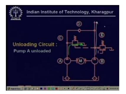
As if the setting is exceeded at some point then what is going to happen is that this relief valve will vent so the pump flow at that time let me use a different color, so the pump flow at that time so this is the case for both pumps loaded so let me go to the other diagram then we will be able to see the case where pump is unloaded. So then when pump A is unloaded because this relief valve setting has been exceeded so this is the flow rate of the pump, right and this so this pump gets unloaded.
