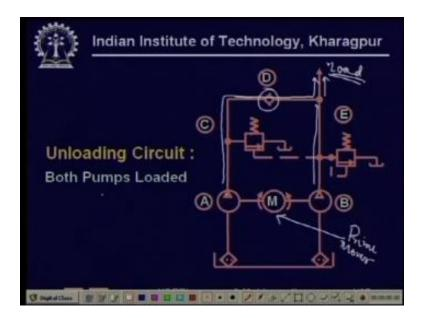
So we first come to our first circuit what is that, in this circuit it is called an unloading circuit so there are see the circuit here are two pumps can you realize that this is actually a hydraulic pump, this is a hydraulic pump this is also another hydraulic pump and they are being driven by a common motor so this is the prime mover, this is the prime mover and this pumps are actually connected in parallel this is where it is going to the load or the system.
