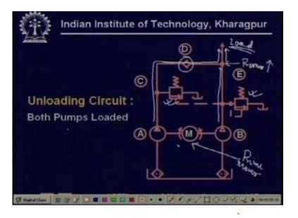
So now we want to the pressure has gone up because the force requirement has gone up so we want to reduce flow rate, so what do we want to do so we have this setting of this relief valve.
