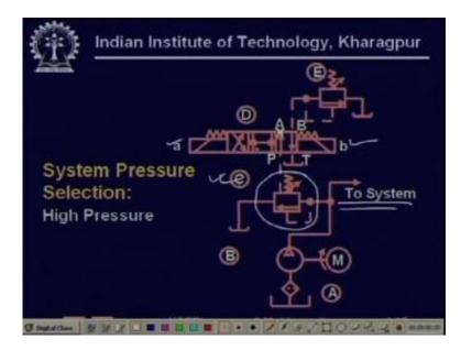
So you see that we are able to achieve this by either energizing A or energizing B or energizing none, so we can select the system operating pressure mode, this is our second example.
