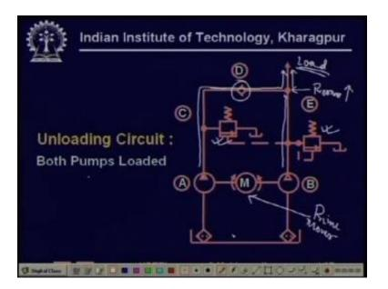
Hydrostatic pumps or positive displacement pump generally so as long as the speed is the same the volume being delivered is the same and the power requirement is directly proportional to the pressure. Assuming that the volumetric efficiency is same the leakage extra are not significant. (Refer Slide Time: 05:29)
