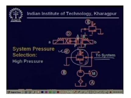
So the operation so now the operation of this valve is not limited by the pilot pressure because the pilot is connected to a plugged port, so the pilot does not vent the valve. So now it is operated by its own setting so now in this system pressure gets limited by the setting of the valve C itself. And since the setting of the valve C is higher than that of E so we can limit the system pressure to a higher level. (Refer Slide Time: 13:54)
