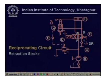
In the next row, now we have a retraction stroke, so what happens is when it reaches the end it operates this limit switch at the end at the extreme end of the extension stroke that limit switch is actually connected to the solenoid in such a way that immediately when the limit switch is made or switched on this solenoid is put off. So, when the solenoid is put off this directional valve assumes the right position so what is happening in the right position.
