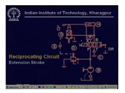
And we have in this case we have only one this thing only one solenoid and the other side is so if you switch off the solenoid it will come to, so it has only two positions.
