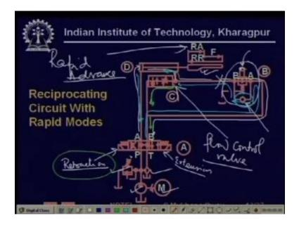
Now what happens when we want to have retraction when we want to have retraction then we will operate this solenoid, when we will operate this solenoid then what happens is now the, let me choose a different color for the blue one so during retraction now this line B is connected to pump so how does it flow, so it flows through this path and this path and this now it flows to the
