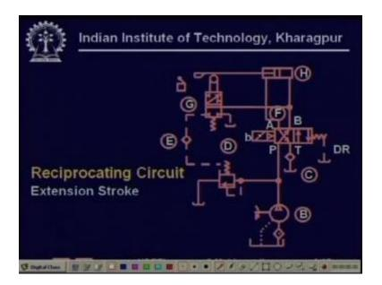
So here is the circuit, so what is happening here very simple again always start from the pump so here is the pump the filter is the drain line, this is the relief valve which is typically used for overload protection of the pump. Now in this case see look at this valve this valve has first of all try to debate the symbol, the symbol has it each has a solenoid plus it has a hydraulic pilot so actually it is a probably this direction valve is actually a very big valve.
