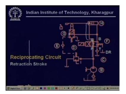
In the right position the pump flow goes like this so now you see what is the matter here, so in the right position the pump flow goes like this and enters what is known as the rod end of the cylinder, so that now the cylinder moves towards the right note that the cam is still not operated so therefore this is still plugged and this is also still plugged and the full pressure is being operated being applied to the cylinder.
