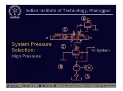
So now we go to the I am sorry, we go to the next one which is the high pressure mode, so what is happening in the high pressure mode, in the high pressure mode we are now in this position, so in this position what is happening first see that this port is actually plugged this is plugged means that it is sealed. So therefore the pilot pressure can go up to any level theoretically speaking can go to very high level.
