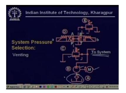
So here is the circuit first for the vent mode, so in the vent mode what is happening look at this circuit, so what components do we have, we have the tank and the reservoir here we have the pump we have the motor we have a relief valve and this is where it goes to the system. Now the pressure limits the pressure upto which the system can occur will obviously be selected by this release valve and this relief valve actually the there are this is a pilot operated reliever valve.
