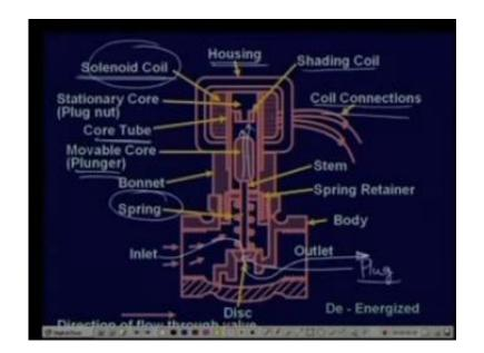
Okay, so right. So what I was saying is that the electro-hydraulic valve pilot stages the solenoid valves are used and this is a particular construction of the solenoid valve. So you see that this is the valve, this is the plug and this is the closed position shown. So this is inlet and is flowing through this and going to this is the flow of fluid, there is a spring loading. Now this is here the stem is actually connected to a to a magnetic core which is called the plunger right.
