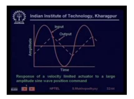
Any actuator most of the electromechanical actuators actually have a rate limit.
