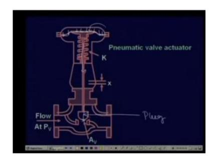
This is on the other hand this is a particular pneumatic actuator so again same thing, again you have a plug and you have these ports. So what happens is that here by spring force this is a particular valve where you can close the valve by applying here in the normal position it will stay open. So there are various kinds of valves efficiency that if you apply energy or force they will close or if you apply energy or force they would be open.
