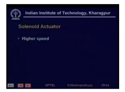
So solenoid actuators have, you know higher speeds they are lower ratings but higher speeds because higher speeds because as we will see that the force on the actuator can be quickly controlled because it is controlled by current. So current can be driven pretty fast, so therefore, forces can be created very fast varying forces can be created and therefore the valve actuation becomes fast.
