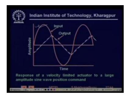
So for example, if you give a large and then high frequency sinusoid then the stem position will not be able to follow it, but rather it will go up like this. So there will be a distortion, you know. So these things are to be kept in mind when one is designing a process control loop with a valve right, that they have these rate limits. (Refer Slide Time: 14:27)
