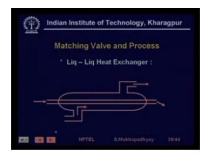
Sometimes you now valve characteristics can be very cleverly used to, you know match the match the system characteristics. So for example, take the case of a liquid to liquid heat exchanger, so what happens is that now, you know this is the input which is the cooling flow and what is the output, the output is the outgoing temperature of the liquid which is being heated let us say.
