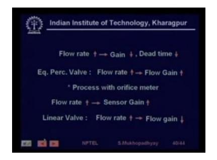
Similarly at the end and an opposite situation can occur if you have an orifice meter, so in an orifice meter as the flow rate increases the sensor gain also increases, so again the loop gain increases, so in such a case the, one has to have the overall gain reducing right. So one can use a linear valve for this.
