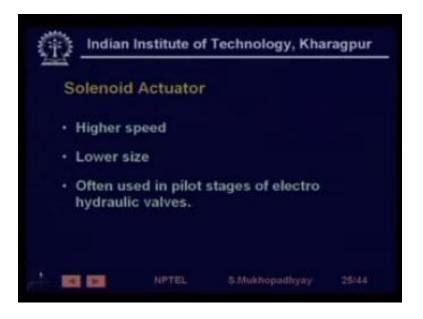
So we are talking about solenoid actuators that they can be used in pilot stages.
