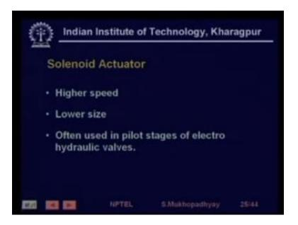
And often they are used as we will see they are often used in pilot stages of electro-hydraulic valve. So you have a big controlled valve and you want to move the valve. So see that big electro-hydraulic valve actually may be controls the flow. Now to move the valve also you need to create you need to move the valve.
