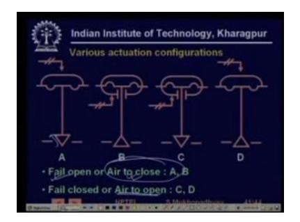
The, lastly you know valves are one has to put a, or have a view towards what will happen if the actuation fails, because you know sometimes this flows can actually cause explosions etc, so valves are constructed in various configurations which are shown here. For example, fail open or air too close. So if this air supply somehow fails then this valve will fail and it will fail in an open situation.
