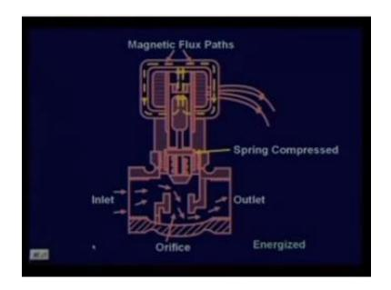
On the other hand when this will, you see that if this is energized then the flux is flowing like this as shown and it is pulling the plunger up. So when the pulling the plunger up then this spring is compressed and this opening is open and the fluid flows. So this is the way our solenoid actuator will work. (Refer Slide Time: 06:08)
