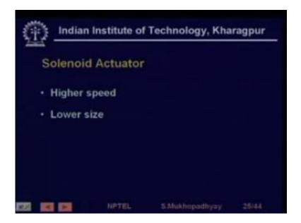
So we have higher speed lower size because pneumatic actuators can be of quite high, I mean of larger size because by just by increasing the diaphragm sometimes we can create a lot of pressure for even higher ratings we can use hydraulics. So solenoid actuators are generally of lower size.
