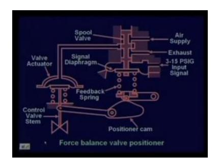
So such a thing is called a valve position and there are various other mechanisms is just one mechanism which we have shown there are various or the flapper nozzle with based mechanisms etc.
