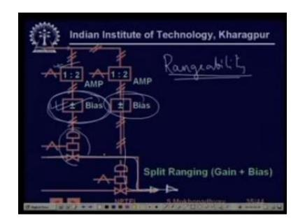
Similarly these are sometimes, you know there is a very important quantity for a valve called a range ability. So range ability means that what is the maximum to minimum flow ratio, so the maximum flow to the minimum controllable flow is it is said. So valves can have you know sometime valve manufacturers claim that they have, you know 10 : 1, 15:1, 13:1, 30:1 kind of you know range abilities.
