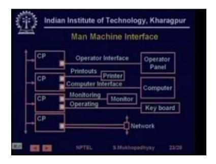
So for example, these are these are so there could be a variety of you know man machine interface kind of devices which needs to be interfaced with a PLC starting from operator panels to monitors 2 pcs to e boards to printers so all these it is it is possible to interface.
