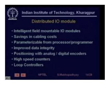
So these are actually intelligent field mountable i/o devices so you actually put the i/o module right there on the machine and from there you draw a wire or you connect it to a network or you take an input-output concentrator and connect several local distributed I/O use and then make one digital communication back to the PLC the advantages are mainly in savings in cabling costs I might have mentioned before that cabling costs are an on a not insignificant part of any
