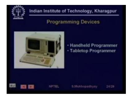
Then you have to have programming devices and this is a typical programmer, programmer a sort of two types either they could be handheld which you can take to the shop floor and directly program the PLC or they could be tabletop where you have which are of higher capabilities and where you actually develop programs offline and maybe go and just load it there because these have very good program development environments also.
