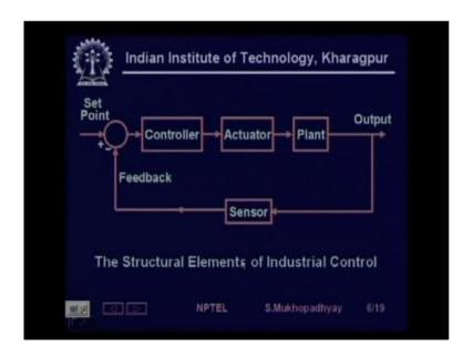
So the structural element so what is basically done in control why do we control we control because we want that the outputs or some process related variables which could be temperature which could be pressure or we want them to behave in certain ways that we desire.
