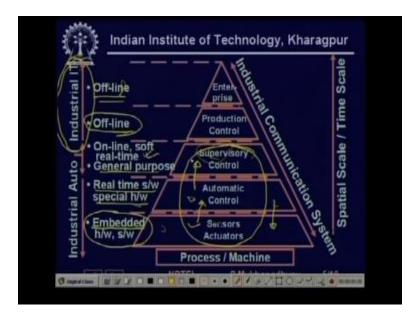
Actuator now similarly the information that the sensors and actuators are that the automatic controllers are receiving from the sensors part of it they are actually passing to the supervisory control layer to see whether the control loop is working satisfactorily or whether some set point change is needed so or whether there is some malfunction some sensor has failed and the process output is going out in which case the Supervisory controller must take some action.
