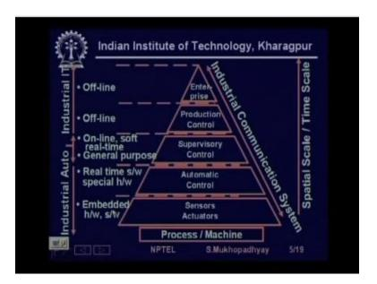
We must understand that much of this technology the much of the part of industrial automation that we are going to concern ourselves with is a is actually about control so we should first see what are the elements of counter of industrial control. (Refer Slide Time: 24:48)
