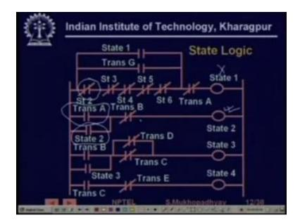
So what happened is that it found that the transition A is on at this point of time it found this transition on because transition logic has been already evaluated and it has been found to be true. So therefore, this auxiliary contact will be closed, so therefore now state 2 will be on. Now once state 2 is on two things happen, firstly you see in the next because state 2 is on this will be on this contact will now be off.
