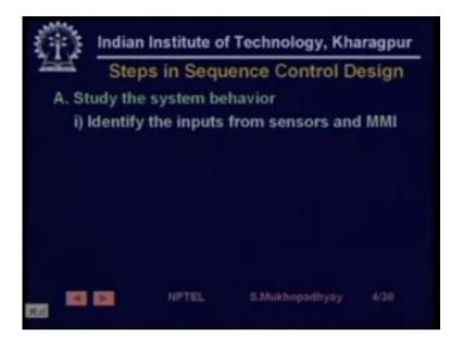
One must first of all identify inputs to this to the system that is the programmable controller program what inputs it will take, inputs can come from either from sensors in the field or it comes from operator interface which I call the MMI or the man-machine interface so somebody presses a pushbutton that is an operator input, right. On the other hand some limits which is made that is a sensor input.
