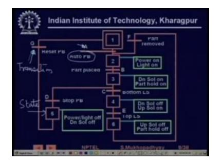
Initially the when you have double square it means that is the initial state, so if initially if the auto push button is pressed this is a transition A which gets activated which will take place and take the system from state 1 to state 2, if the auto push button is pressed so this is the transition condition. You can have much more complicated conditions in this case we have very simple conditions.
