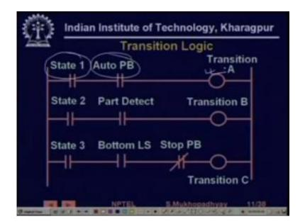
And at that point of time if the auto push-button signal comes then transition A will get enabled, so it will be on right, so if you have modeled if you have model or system well then at a time only one transition will get on right, if you have if we do not consider concurrency then at a time only one transition will get on. Now what will happen, now in the next stage so now transition A becomes on and state 1 was already on, so at this point of time we come to the state logic.
