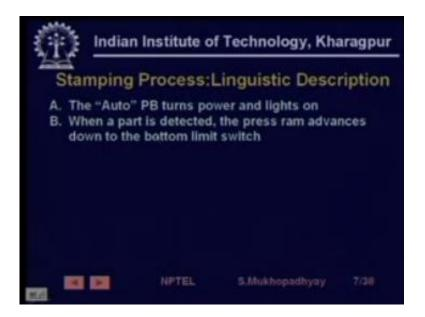
Where a part is detected the thing to be stamped when it is detected which one is placed at the proper place and detected, so there has to be a part sensor. The press ram the thing that will the heavy piece which will move and make a stamping it advances down.
