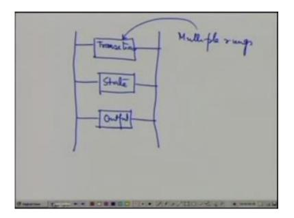
So the relay ladder logic will consist of three different blocks, okay. The first block will contain the transitions this is multiple runs then the state block and finally the output block, so we will now describe these three blocks in the case of this example. (Refer Slide Time: 18:22)
