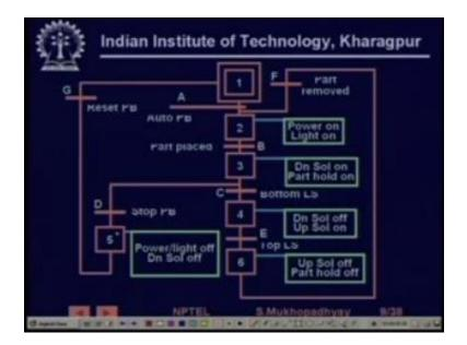
So what is happening in this diagram is that let me select my pen, so what is happening is that you see these squares are the states, we are possibly familiar with state machine so a state machine is like a graph which consists of a set of states these squares are the states. (Refer Slide Time: 12:22)
