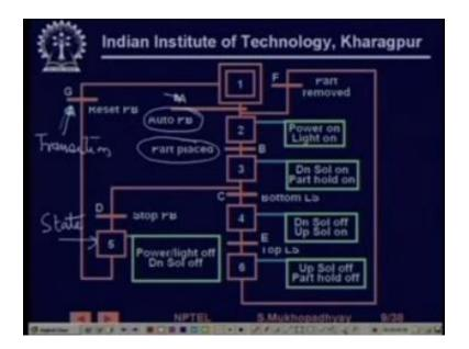
And then if this transition occurs then the system comes to state 2, in state 2 again if this transition B takes place whose condition is part placed it will come to state 3 so in this way depending on how the sensors are bringing in signals from the field the various transitions will be enabled and the system will hop from state to state that is the behavior of the system.
