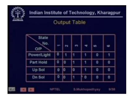
And these are the outputs which are exercised at different and that is actually also encaptured in what is known as an output table, so the output table says that among the four outputs that we have namely power light, part hold, power lights which part hold up solenoid and down solenoid. Which are what are the status whether they are on or off in the various state so there are six states and there are four outputs so it says that the power light switch stays on in state 2, 3, 4 & 6 right.
