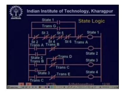
So now let us see what happens in the state logic, in the state logic see state 1 was on, right now because state 1 was on and because auto push button was pressed transition A became on, so the computation came from the transition logic to the state logic, so what happens is that it found state 1 is on.
