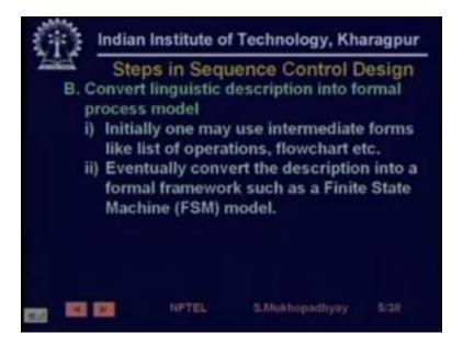
Then finally, but finally it is prescribed that one should be able to convert it to a formal mathematical framework something like let us say a finite state machine which we will be using here, after up to this the operations are manual having done that then one has to go for design of the sequence control logic based on the formal model.
