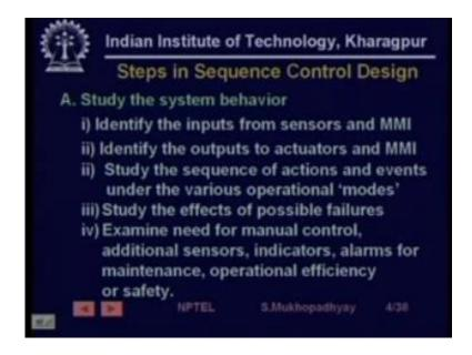
Then even apart from the automated behavior one has to examine the requirements that exist for number one manual control, manual control is very important because for finally if the automation equipment fails it should be able to operate the system using manual control, right maybe right on the field while the automated control may be actually working quite a distance away from the actual equipment it may be housed in some control room.
