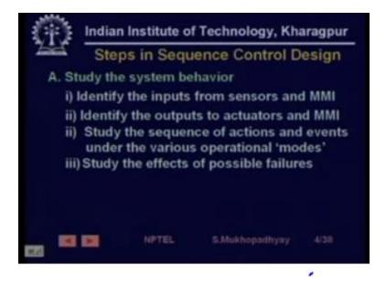
Then one thing that must be very clearly remembered is that when you are developing and an industrial automation program one not only has to remember, not only has to design for normal behavior but one must to some extent at least take into account the possible failures that can occur, otherwise a system that behaves well under normal behavior can behave in a very nasty manner if some simple element of the system like a sensor fields, right.
