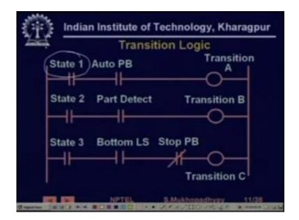
So it says that if the system is in state 1, if it is in state 1 that depends on the state logic then the corresponding to the state corresponding to every transition we have an output coil and corresponding to every state we have output coils. So this is actually an auxiliary contact corresponding to the output coil called state 1, so it is an abstract variable actually so it says that if it the system is in state 1 then this contact will be made.
