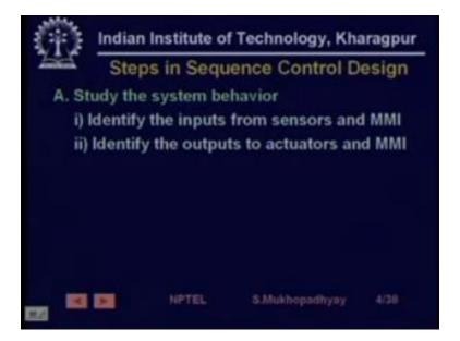
Similarly identify the outputs, so switch on motor, so motor is an actuator that is a kind of output there is another kind of output for example, switch on some indicator or some lamb that would be an output which again goes to the MMI or the man-machine interface. So we have to first identify these.
