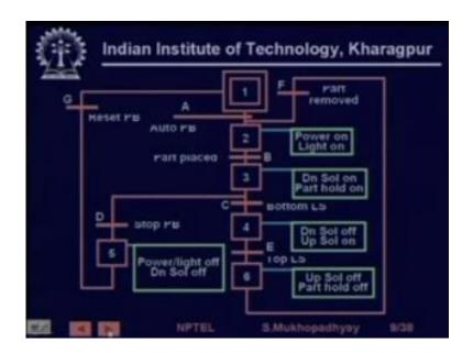
We could go back just for once so you see here transition A takes the system from state 1 to state 2, transition B takes it from state 2 to state 3, transition C and D are in parallel it could take state 3 to either 4 or 5.
