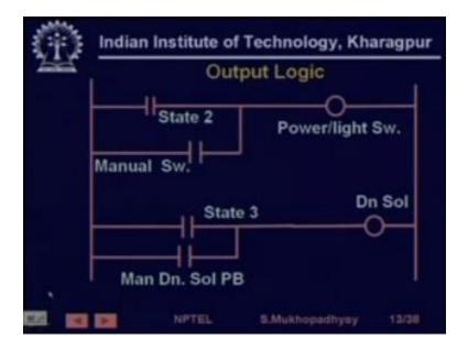
So we can this is just to demonstrate that you can put additional logic to include manual operation of the system. So in this, so otherwise this program simply says that while you are in state 3 down solenoid will have to be activated very simple.
