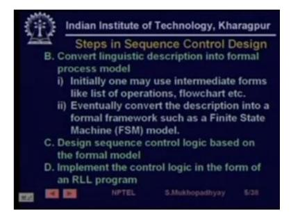
And then finally one has to implement the control logic in the form of an RLL program and it is preferable that these steps especially the step D is made as much as possible automatic, because this is a step which can be done in an automated manner once B and C have been carried out and for large programs it is always preferable to go for automatic programming because that will always lead to error-free programs provided your specifications were correct.
