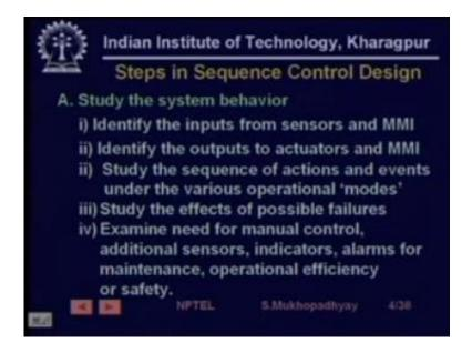
Indicators alarms and as well as operational efficiency or safety these are the factors which must be considered to finally arrive at the functionality, one must always remember that the customer may not always be able to express his or her needs and a good automation engineer should be able to supplement it with his own experience in such cases, so having done that the next step is to convert. (Refer Slide Time: 06:04)
