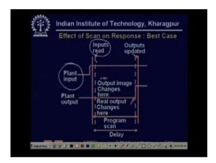
We remember that the plant input can change at any arbitrary period of time we cannot control that right so suppose the plant input change is just before and in the inputs are red so then immediately after it changes it will be read that is this change will be reflected and will come to the processor IO image very quickly.
