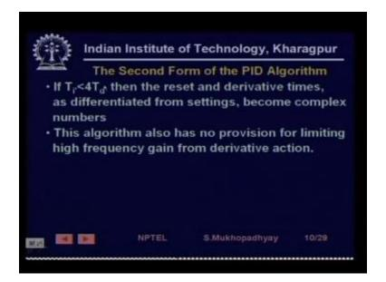
In the second form where Ti' is less than equal to 4Td' if you want to say it you actually cannot set it in the first form because it turns out that that if Ti' is less than 4Td' then Ti, Td values are complex they are not they are not you would not get real numbers TI and TD which will be able to realize this. So you see the first form is somewhat constrained, on the other hand the second form in the second form.
