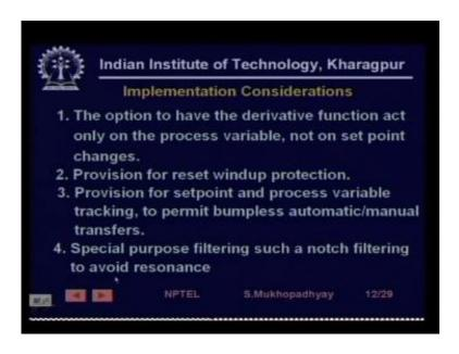
Somewhat like this you know so in this range they will pass control signals in this range also they will pass control signals but in this narrow range they will stop the signal, so if you have your resonant frequency in this range this is omega this is say U Omega J Omega so in this range this one this notch filter other is this is actually gain of the notch filter so it is GJ Omega so in this range the notch filter will not allow any inputs to come. (Refer Slide Time: 28:27)
