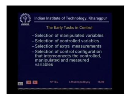
Selection of control configuration that is how you are going to connect the controllers and the sensors are you going to connect it in cascade with feed-forward or you have seen some special features like you know Smith predictor so these needs to be need to be done.
