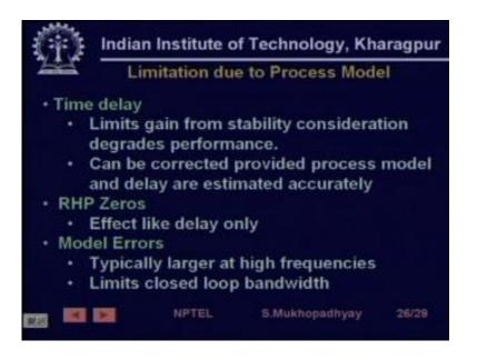
Half-plane zeros are like delays and model errors so remember that models model errors are always high in the high frequency zone so increasing the bandwidth you are going into the uncertain soon. (Refer Slide Time: 55:42)
