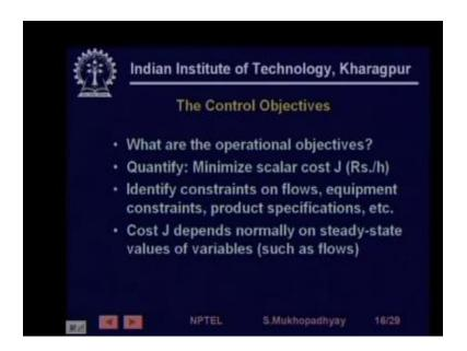
It turns out that costs j that is the cost that you want to minimize depends generally depends much more on steady state values of variables especially in process control such as flows because process controls are not processes are typically not always not all the time oscillating right they will they will oscillate once in a while but most of the time they are going to stay you know in their steady state and therefore it is the steady state values which are which mainly decide the cost.
