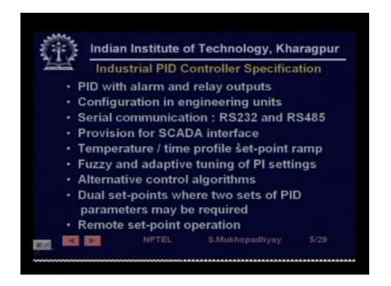
So let us first look at an industrial PID controller specification, this is a very typical specification, this one is adapted from a Honeywell PID controller which is very, very and well it is a standard company very well known company in the field of process control. So we first have, we have several features first with that you have it says that you have PID with alarm and relay outputs.
