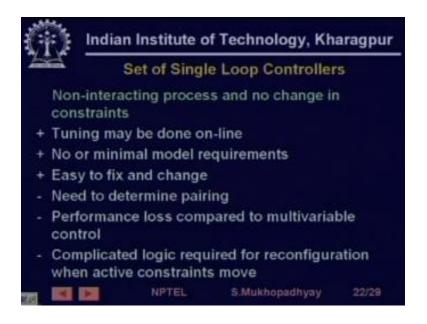
Similarly it turns out that you have performance loss you cannot achieve such control such good control as you can with multi variable control and when we have active constraints then you have you have very complicated logic you must have above these set of single loop controllers you must have supervisory logic which will look at all these single loop control as and probably carefully manipulate the set points.
