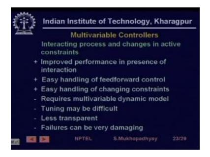
Significantly improved performance in presence of interaction you have easy handling a feed forward control again feed forward is you know tends to make the system multivariable you have easy handling of changing constraints as we have mentioned and it requires a multivariable dynamic model tuning is obviously difficult much more difficult than a set of single loop controls difficult to understand less transparent and this is important thing that that failures can be very damaging.
