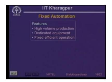
So for example the LSA the blast furnace or the steel melting furnace or the continuous caster these are equipment which are likely to have a long life so and they handled so much of equipment so much of it so much of material so much of energy that it makes sense to make them very tuned for efficient production so factory types are typically. (Refer Slide Time: 16:36)
