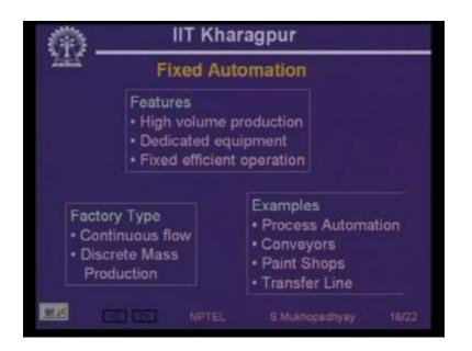
Automation controls for these kind of you know steel oil refinery kind of things for example there are parts of automation which do not need to be changed when there is not much to change it for example conveyors main nearly same always so that is the fixed automation paint shops generally painting is that you need to put the object at one place and you not be you need to jet spray it the paint so the operation itself is simple does not is not likely.
