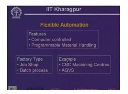
So the examples are CNC machining centers and guided vehicles automatic guided vehicles now still all these that is fixed programmable and flexible they are mainly concerned with automation over a limited special range so you are talking about local automation maybe within a shop or maybe within parts of a shop or maybe involving just one or two machines, now if you want to really control the whole factory in a in a very integrated manner and in a very optimal manner.
