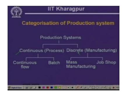
So again continuous processes could be divided into two kinds one are called continuous flow processes typically means that a product is manufactured for a considerable amount of time and continuously a the product manufacturing goes on like the case of let us say oil refineries or the case of steel plants very big factories manufacture maybe four or five kinds of products may be let us say gasoline petrol kerosene these are typical product types of a refinery. Similarly you could have a batch.
