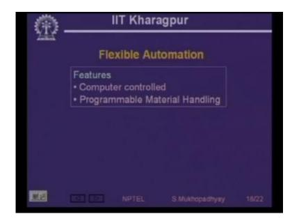
Should be also programmed because if the sequence changes then parts will have to travel from one place to another and so if you use material handling equipment for which is fixed then you cannot transfer parts from one place to another very flexibly that is why you need programmable material handling so factory types are job shops .
