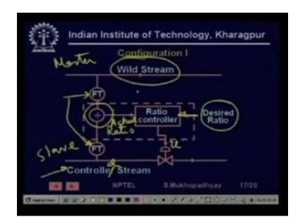
So the first one is configuration one let us see that, so you see in ratio control we have two streams, the first one we can recall the wild stream. So we do not directly control that stream, that stream is controlled by other considerations may be from production volume words. but so it is like a master stream which changes independently because of some operator change etc. And this is the slave stream or the controlled, this is not controller, this is controlled stream.
