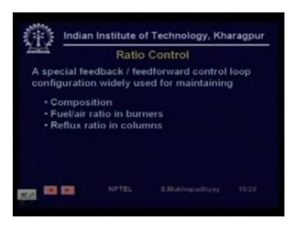
Similarly in distillation columns reflux ratio is a very important thing which decides product quality. So there are various situations where two materials must be must be brought together in some reactor or some chamber in precise volumetric flow ratios right. It is in this situation that you apply ratio control, there are two typical configurations in which ratio control is used.
