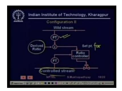
So you are saying that you measure the flow rate in the wild stream, if you multiply by the derived ratio what we will get, you will get that at this flow rate of the wild stream how much of the control stream material should come. So in that sense it is a set point for controls for the flow rate of the control stream.
