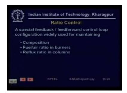
So it is a special feedback feed forward control loop configuration which is widely used for maintaining composition control, fuel air ratios in burners. For example, let us say if you have a any kind of burner let us say a boiler, so boiler the furnace. So you have to produce flame, for producing flame you need two things you need the fuel and you need the air, but they must be provided in such a ratio such that complete combustion takes place.
