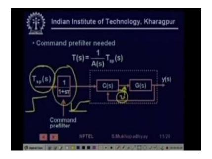
So if we have step like set points therefore we often put what is known as a command pre-filter by in which what we what we do is that we don't not allow the operator to give the set point directly to the plan but we put a filter in front, so that even if he gets give the set point the actual set point which will go to the plant will rise slowly so in such a case this control input saturation U saturation will not take place and you can still control it.
