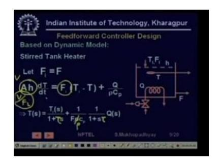
Feed forward controller design based on a dynamic model so again the same process again the same equations now so obviously if you take if you take Laplace transform then you will get a model like this here this should be Rho this is wrongly typed this should be Rho this is tau the
