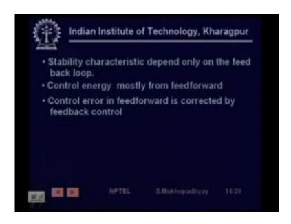
So now we are making some comments first thing we says that the stability characteristic depends only on the feedback loop obviously because the feed-forward loop does not it is a kind of open loop so there is no stability question here but the control energy comes mostly from the
