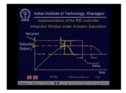
The control input is now reduced now what is going to happen what will be observed is that the while the why it would have been desirable that the control input immediately falls down and reaches as reaches the desired steady state point it does not do that rather it continues at the same level we ignoring that the set point has now been reduced and overly after some time only after some time does the actuator does the.
