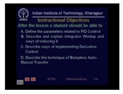
One technique of you know bump less auto manual transfer that is when the control is transferred from auto to manual or manual to or to how so that it can happen without any shock to the process and finally we will describe digital implementations.
