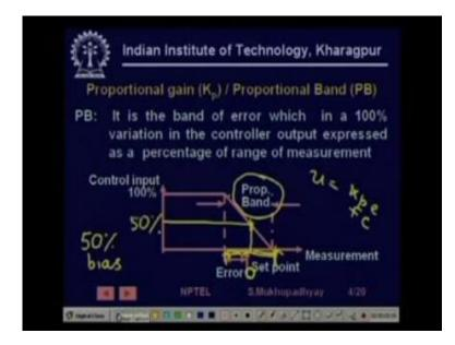
So look at this diagram will clarify matters further so here look at the controller input and suppose this is the set point currently the set point is set here okay so if the measurement or the output is the measurement of the output could be anywhere in this zone so for very so it will cause various kinds of error and if you use a proportional band then as the error will increase the output will increase in this case the proportional controller actually has a 50% bias which means that.
