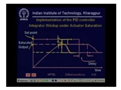
Control start respond to the stage to the set point now this phenomenon is called integrator windup basically what has happened is that the integrator has become bloated or floated so it has not realized that the plant cannot reach this output so the error is will persist so it is unnecessarily trying to give more and more control input and getting blown up right so that is integrated windup and it happens essentially because of the fact.
