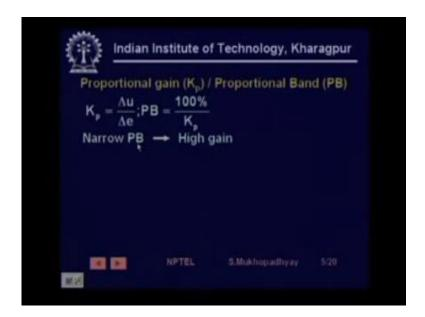
So while KP is  $\Delta u / \Delta e$  proportional band is defined as one hundred percent by K<sub>P</sub> so you can easily find out that this gives the error in percentage which will cause a 100% input change obviously an arrow K<sub>P</sub> means low value of K<sub>P</sub> implies a high value of get an arrow.
