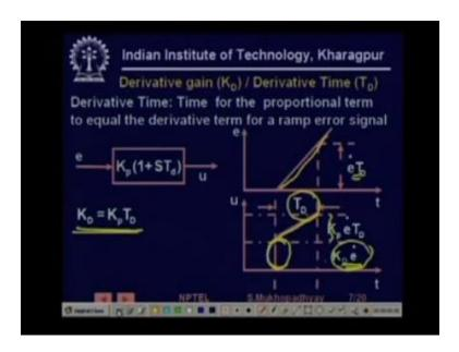
And we have a derivative time so again now the derivative time is the time taken for the proportional term to equal the derivative term for a ramp error signal so again a similar thing so let us look at the diagram here so here now we have a PD controller right so in the PD controller if you feed it a ramp signal now let us say a ramp signal of some slope e dot some slow e dot then immediately what will be now that now the derivative term will jump because there is a constant e dot.
