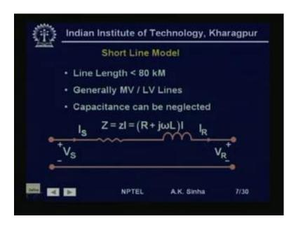
Now, transmission lines which are less than 80 kilometers long or about 50 miles long, we neglect the effect of capacitance. Because, the capacitive effect or the charging current is not very large and it is effect can be neglected. Also these lines are generally medium voltage and low voltage lines, because these are very short lines. And therefore, also the charging current, because the voltage being small will also be much smaller.
