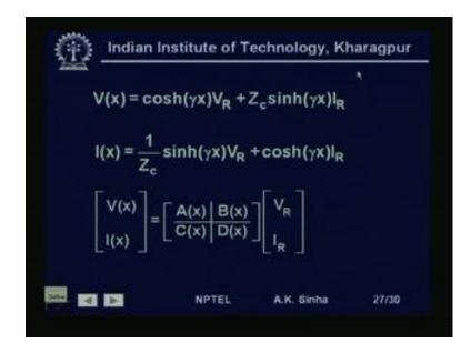
Now, from this we can ((Refer Time: 47:46)) this term e to the power gamma x plus e to the power minus gamma x by 2 is equal to cos hyperbolic gamma x. And e to the power gamma x minus e to the power gamma x by 2 will be equal to sin hyperbolic gamma x. Therefore, we have this cos hyperbolic gamma x into V R plus Z c into sin hyperbolic gamma x into I R, that is what we get here.
