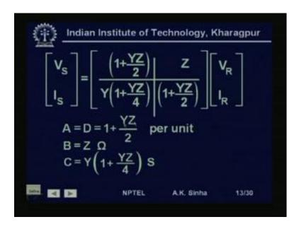
In terms of ABCD parameters as V S is equal to 1 plus Y Z by 2 V R plus Z I R, I S is equal to 1 Y into 1 plus Y Z by 4 VR plus 1 plus Y Z by 2 I R, which shows that A is equal to D, that is A is equal to D is equal to 1 plus Y Z by 2 this will be in pi unit. B will be equal to Z ohms and C will be equal to Y into 1 plus Y Z by 4 Siemens. So, for a medium length line, when we are using a nominal pi equivalent for this medium length line, we have the ABCD parameters.
