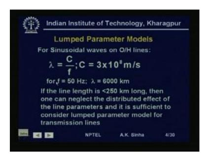
What we will see is that for sinusoidal voltage and current waves on overhead line. The wavelength of the line is given by this lambda; wavelength of the line is given by C by f, where, C is the velocity of light or the velocity of propagation of the waves, current or voltage waves on the transmission line. For overhead transmission line, this will be very nearly equal to the velocity of light.
