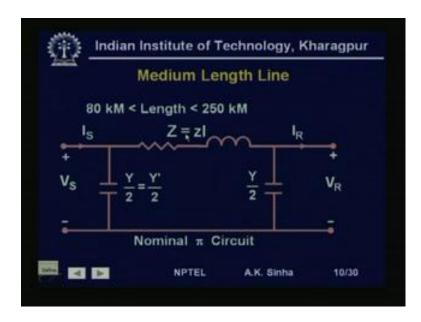
What we do here is, again we are use a lumped parameter model where the complete series impedance that it is total resistance of the line, is lumped as one resistance. And the total inductance of the line is again lumped together. So, we get this R plus j omega l as the series impedance of the line. So, Z the total series impedance is equal to z into l, where small z is the series impedance of the line per unit length.
