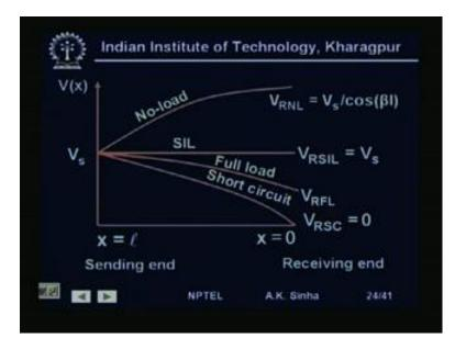
When we have a surge impedance loading. The voltage across the line all along from the sending end to receiving end is going to be same. If the line is unloaded, then the sending end voltage.
