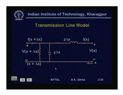
For this line of a length delta x, we have the transmission line impedance. Or the series impedance of the transmission line, which is given by z into delta x. It consists of the resistance of the line and the inductance of the line. These will be per unit length or per meter multiplied by delta x will give us the value of series impedance, z delta x for the delta x length of the line.
