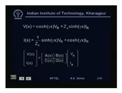
Now, here if you see A x is equal to D x and that is equal to cos hyperbolic gamma x in per unit. That is if you see this relationship this is your A x and this is your B x, this is C x and this is D x. So, A x is equal to D x is equal to cos hyperbolic gamma x B x is equal to Z c sin hyperbolic gamma x, V x is equal to Z c sin hyperbolic gamma x. C x is equal to 1 by Z c sin hyperbolic gamma x and D x as we have all ready seen is equal to A x.
