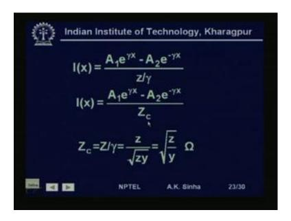
So, I x is equal to A 1 e to the power gamma x minus A 2 e to the power minus gamma x divided by z. And the gamma which was here multiplied with A 1 and A 2 that we have taken on in the denominator, so this is z divided by gamma. Therefore, we can write I at x is equal to A 1 e to the power gamma x minus A 2 e to the power minus gamma x divided by Z c. Now, this term z by gamma we are writing this as Z c, Z c is called a characteristic impedance of the transmission line.
