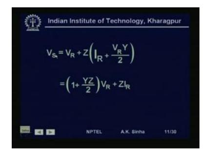
And we can use the ABCD parameter for this as V S, from here we can see is equal to V R plus Z into I R plus V R into Y by 2. Now, if you look at this circuit, what we are finding is, V S this voltage will be equal to the drop in this. Now, what will be the drop in this, this drop will be equal to how much current is flowing in this part IR plus VR into Y by 2.
