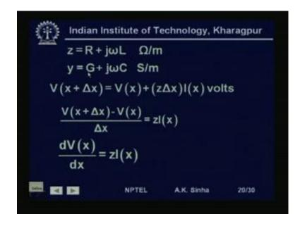
Here, we have V plus V at x plus delta x will be equal to V x. That is the voltage at distance x plus the voltage drop, that is the voltage drop here will be I x into z delta x. So, the voltage at this end, that is V at x plus delta x is going to be equal to V at x plus the voltage drop, which is I at x into z delta x. That is what we have written here, V at x plus delta x is equal to V at x plus z into delta x into I x I at x.
