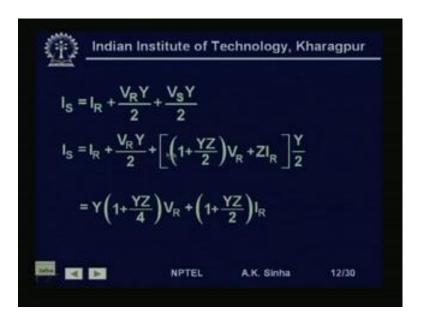
So, we are writing I S is equal to I R plus V R into Y by 2 plus V S into Y by 2. Now, again rearranging this by combining terms, we write this as I R plus V R into Y by 2 plus V S. We are writing the relationship for V S from the previous equation here, V S is equal to 1 plus Y Z by 2 into V R plus Z I R. So, substituting this value for V S, we are putting it here, so V S into Y by 2 we write here.
