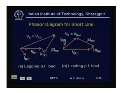
The Phasor diagram for short line can be developed, we can start with the voltage at the receiving end at full load. So, V R f l as the reference voltage and we have a current I R at full load, which is in this direction, that is lagging the voltage by some angle theta. Now, with this we can find out using the circuit model, voltage at the sending end, which will be equal to V R f l plus R into I R f l.
