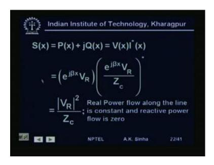
See this relationship, the voltage that is the power flowing is proportional to square of the voltage. So, if you are doubling the voltage, you are able to transmit 4 times the power and so on. Now, I will show you the characteristics of this long lose less transmission line.
