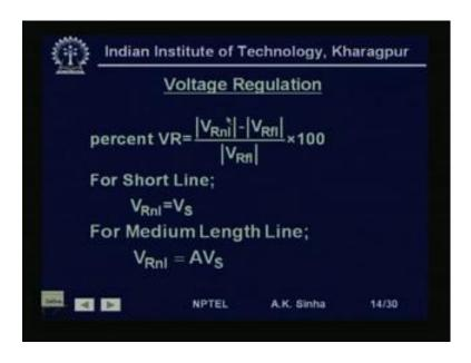
So, percent voltage regulation is defined as V R no load minus V R full load divided by V R full load into 100 percent. So, this is what we define, basically what we are trying to say here is that suppose we have a line which is loaded to it is full load value. And if the load is suddenly thrown off what will be the voltage at the receiving end. How much rise of voltage is there at the receiving end.
