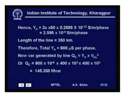
Hence, we can calculate the admittance Y n is equal to twice pi f which is 50 into the C. This is C n that is 8.2595 into 10 to power minus 12 Siemens per meter per phase, this is equal to 2.595 into 10 to power minus 9 Siemens per phase. Now, length of the line is given as three 50 kilometers, therefore total admittance will be simply multiply this by 350, this conserved to be 908 micro Siemens per phase.
