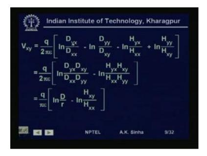
We can write this voltage from the earlier lesson, that we have had. We can write this voltage V x y is equal to q by twice pi epsilon into log n D y x. That is the distance of the conductor b to conductor a divide by D x x. That is the distance of conductor a to conductor a, that is conductor x to conductor x. So, in similar way we will write for the charge on conductor y, considering the charge on conductor y.
