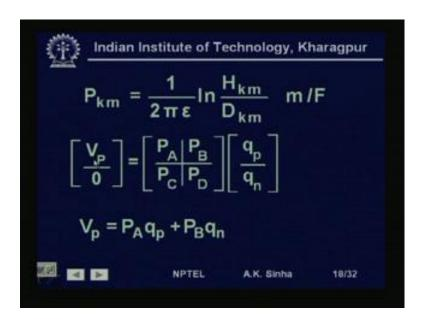
Here P k m, that is any of these terms P k P a b P b b or P n 1 b. Any of these terms, is given by the relationship 1 by twice pi epsilon log n H k m by D k m meters per farad. Now, this matrix which we had this big matrix relationship can be written in a shorter form as V p which is the voltage for the phase conductors. And 0 which is the voltage for all the n ground conductors is equal to P A, P B, P C, P D which we had already defined earlier.
