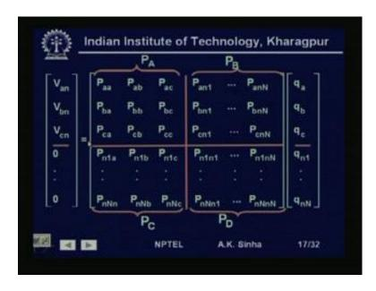
Now, we can put this whole equation into a matrix form as shown here. V a n, V b n, V c n and V n 1, V n 2 and up to V n N, these are 0's is equal to a matrix of P's into q a the charge on conductor a. Q b the charge on conductor b, q c the charge on conductor c. Q n 1 up to q n N the charge on neutral, conductors or the ground conductors which are placed above the phase conductors. That is we are talking about the charges on these ((Refer Time: 34:15)) conductors, n 1 n 2 up to n N.
