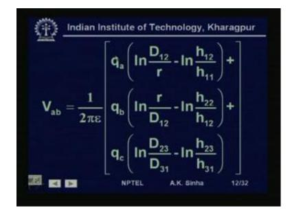
Now, we can calculate the voltage between 2 phase conductors. So, we will calculate that voltage V a b, the voltage between conductor a and b. And this will be given by 1 twice pi epsilon n 2 q 2 charge on conductor a, that is q a. It will be log n D 1 2 by r minus log n h 1 2 by h 1 1, ((Refer Time: 22:02)) that is log n D 1 2 by r. That is from this conductor distance of this from phase b conductor D 1 2.
