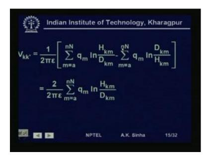
Now, for this system, again we can find out the voltage between any conductor and it is image. That will be given by V k k dash. For any conductor k, we can write the voltage between the conductor k and its image k dash. That will be equal to 1 by twice by epsilon, summation of m is equal to a to n N, where n N is the total number of conductors in the system into q m, the charge on conductor m log n.
