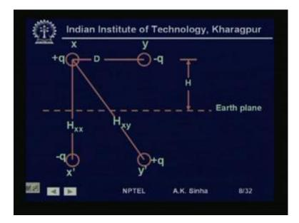
Now, here we have a single phase line with two conductors x and y. Placed at a distance D, the conductors have a radius of r x and r y. The charge on conductor x is q coulombs
