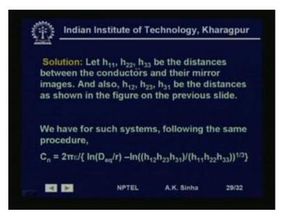
So, we have seen that h 1 1, h 2 2, h 3 3 is the distance between the conductors and their mirror images. That is h 1 1, this should be h 1 1, from this conductor to this a to a dash is the distance between image conductor this will be a 40 meters. Similarly, b b dash will be forty meter and c c dash will be 40 meters. So, and h i j as we have said is the distance shown in the figure.
