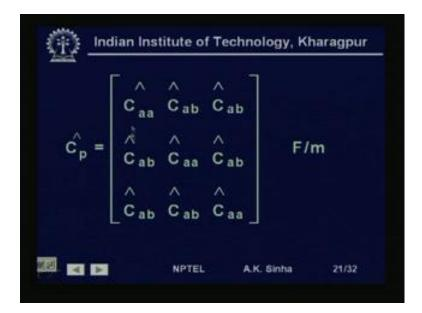
Therefore, C a a hat is equal to C b b hat and will be equal to C c c. So, the three will have the same capacitance to neutral, whereas C a b and C b c will also be same. So, we are for a transpose line system, we are representing them with hat which shows that. This line is a this capacitance is for transpose line, not to confuse with the capacitance that we had calculated earlier.
