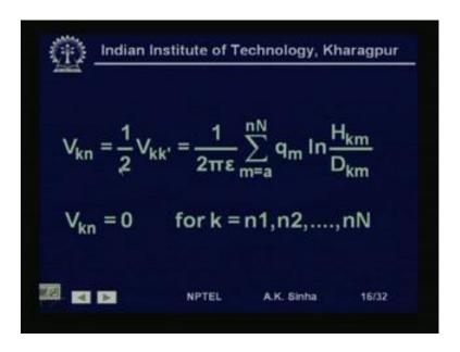
Now, the voltage between the k th conductor and the neutral, or the earth will be equal to half of that between the conductor k and it is image k dash. Therefore, V k n will be equal to half V k k dash which will be equal to 1 by twice pi epsilon. Because, that 2 is cancelled out with this 2 here. So, it is 1 by twice pi epsilon summation m is equal to a to n N of q m log n H k m by D k m.
