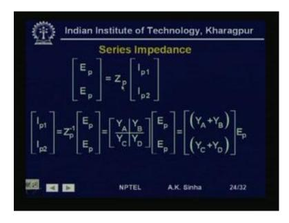
Now, for the two circuits we can write, the relationship E p 1 is equal to Z p 1 into I p 1 and E p 2 is equal to Z p 2 into I p 2. But, since these two circuits are close together there is mutual coupling. So, it will not be right to write separate equations for the two. In fact, what we have here is we are considering a system of 6 conductors, instead of 3 conductors.
