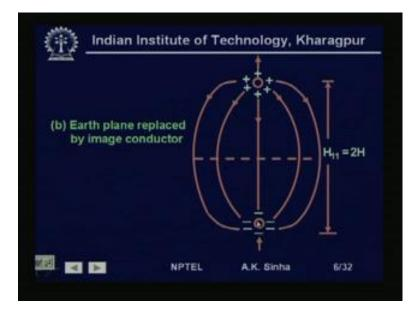
Now, in this what we do is, we consider a conductor directly below the overhead conductor in the ground at a distance; which is equal to the height of the conductor above the ground. That is we are considering an image of this conductor below the ground. So, this is a mirror image of this conductor. And the charge on the image conductor is opposite of that of the overhead conductor. Now, if you see, if you have such a system, then the field lines will look like as shown here.
