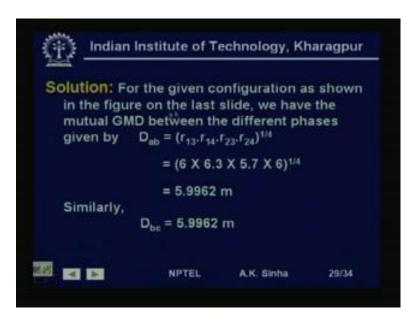
So, for this system, what we have to do is, we have to find out the equivalent distances. So, for the given configuration as shown is figure, we have the mutual GMD between the different phases given by D a b is equal to r 13, r 14, r 23, r 24. That is distance from here to this conductor, distance from this to this conductor, distance from this to this conductor.
