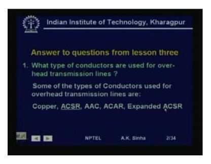
First question was, what are the types of conductors used for over head transmission line? Well, some of the types of conductors used for over head transmission lines are copper conductors, which is very rarely use nowadays. ACSR, that is Aluminum Conductors Steel Reinforced conductors. Then, all aluminum conductors are ACAR conductors or expanded ACSR conductors, which are used.
