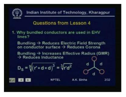
I would like to answer those questions. That I ask in lesson 4. First question was, why bundle conductors are used in EHV lines? Well, the answer to this question is bundling of conductors. That is, instead of using one single conductor, use of a number of conductors connected by conducting frames, reduces electric fields strength on conductor surface, which in effect reduces the corona losses, which result in power loss.
