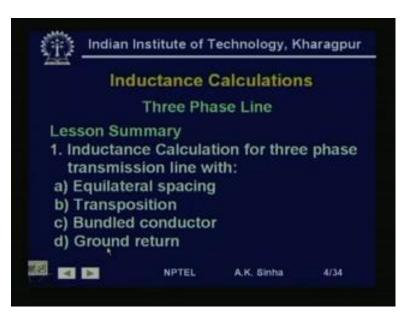
Now, we will start our lesson 4, which will be on inductance calculations for three phase transmission lines. Well, in this lesson, we will discuss inductance calculation for three phase transmission lines with equilateral spacing, then with transposition. Again, with, when we are using bundled conductor lines and finally, lines with ground return. Well, first, we will take the calculation of inductance for a 3 phase line with equilateral spacing or equal spacing.
