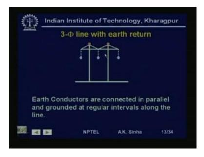
Now, we will take up three phase line with earth return. Now, this is a normal situation. Those three conductors may be horizontally placed and we have at the top of the transmission tower earth wires or the ground wires. These ground wires as I have said earlier in lessons 2. That these ground wires are used to protect the phase conductors from direct lightening stroke.
