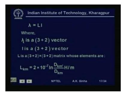
Since, lambda is equal to L I, where L is the inductance and I is the current. Now, in this case, since there are five conductors, we have lambda for all the five conductors. That is lambda a, lambda b, lambda c and lambda n 1 lambda n 2. So, lambda is a 3 plus 2 vector, I again, since the current is following in all these five conductors. So, I is a 3 plus 2 vector.
