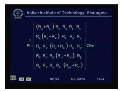
Here, the matrix R is a 5 by 5 matrix and this is represented by for R A a, what we have is, R a plus R k dash. That is this is for R a, the resistances for conductor A. Now, R k dash is the resistances for the image conductor, which is below A. Then, we have R k dash for the other 4. Similarly, for R will be R 12 will be R k dash R 2 with 2 will be R b plus R k dash R 23 will R k dash and so on. So, this is a 5 by 5 matrix, which is a resistance in ohms per meter for this five conductor system.
