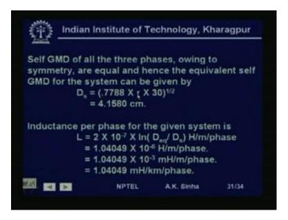
Now, the self GMD of all the three phases point to symmetry are equal. That is, the self distance each conductor has the same radius and the distance between the two conductors of a bundle is same. That is 30 centimeter. So, therefore, the D s for each phase conductor is going to be equal to r dash. That is 0.7788 into r for the conductor into 30 centimeter, which is the distance between the two conductors of the same bundle.
