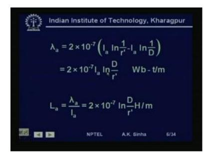
Now, we know that, for a 3 phase three conductor line I a plus I b plus I c is equal to 0. Therefore, I b plus I c is equal to minus I a. Therefore, we can write lambda a is equal to 2 into 10 to the power minus 7, I a log n 1 by r dash minus I a log n 1 by D, which results into 2 into 10 to power minus 7, I a log n D by r dash Weber turn per meter.
