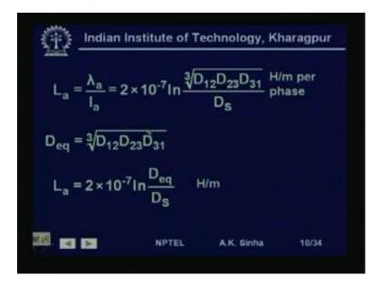
Now, once, we have got the flux linkage, average flux linkage, we can get the inductance, average inductances per meter. Length of the line as lambda a by I a, which turns out to be 2 into 10 to power minus 7, log n cube root of D 12 into D 23 into D 31 divided by D s. Where, this term cube root of D 12 into D 23 into D 31 is called the equivalent distance of the three phase system.
