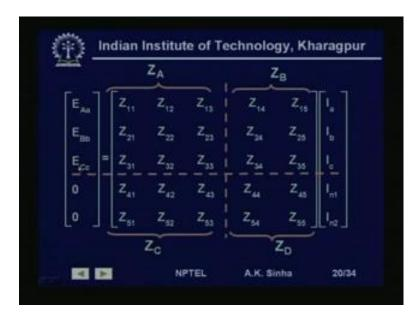
Now, if you write the complete system equation for the voltages across the line conductors. Then, we will have the voltage as E A a, E B b, E C c. That is the voltage across the two points of the phase A conductor, phase B conductor and phase C conductors. Similarly, for the neutral conductors, since the neutral conductors are grounded, this voltage will be 0.
