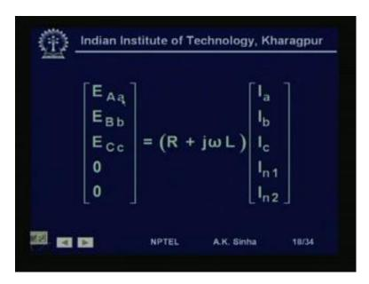
And therefore, we can write this as matrix equation, where we are saying E A a is the voltage drop in phase A conductor. E B b is the voltage drop in phase B conductor. E C c is voltage in phase C conductor. For the neutral conductors is there are grounded, there potential is 0.
