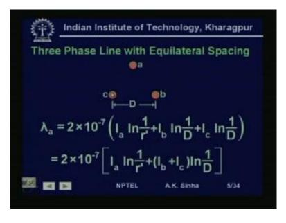
Now, here in this diagram, you can see a, b, c are the three conductors, which are placed at the vertices of an equilateral triangle. That is the distance, among all three conductors are same. That is distance D. Now, if we calculate the flux linkage of conductor a, due to currents flowing in conductor a, b and c. Then, it will be equal to 2 into 10 to power minus 7 into I a log n 1 by r dash, where r dash is the effective radius of conductor a.
