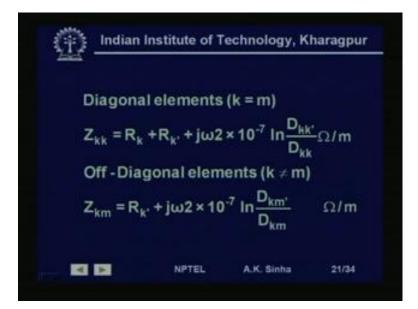
That is Z k k, which means Z 11, Z 22 and so on are given by R k plus R k dash plus j omega 2 into 10 to power minus 7, log n D k k dash by D k k ohms per meters. Whereas, these are the distances, as we have seen in the system in the system diagram earlier. Off diagonal elements that is Z k m, which is basically Z 12, Z 13 or Z 54, all these off diagonal elements.
