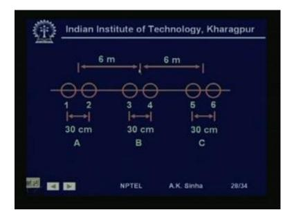
That is, we have a 30 centimeter bundle spacing for the conductors and each conductor as a radius of 0.74 centimeter. The distance between the two phase conductors is 6 meters. That is from center to center. And this is a horizontally spaced configuration. The line is fully transposed. For this line, determine the inductance per phase in milli Henry per kilometer and in milli Henry per meter. Find the inductive line reactance per phase in ohms per meter at 50 hertz.
