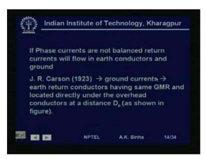
So, if phase currents are not balanced, return currents will flow in earth conductors and ground. Because, since these earth conductors are connected to the tower and again, there are grounded by the footing, ground tower footing. So, the current flowing in these earth conductors will go into the ground. And will this disperse and flow in the ground also.
