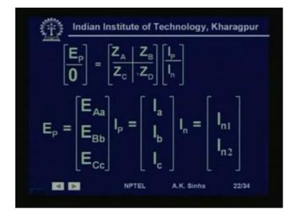
Now, what we can do, since we have already divided this system into four sub matrices. Now, we can write this whole system of equation in a short form like E p, where E p is the voltage drop across the face conductors, 0 is the voltage drop across the neutral conductor, this is equal to Z A, Z B, Z C, Z D into I p. Where I p is the current flowing through the face conductors and I n is the vector of current flowing through to neutral conductors.
