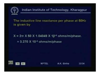
The inductive line reactance per phase at 50 hertz is given by x is equal to 2 phi f into the inductance. So, this is 2 phi 50 into 1.04049 into 10 to power minus 6 ohms per meter per phase. This comes out to be 3.270 into 10 to power minus 4 ohms per meter per phase. So, this is, how we can calculate the inductance and the inductive reactance for any given three phase transmission system.
