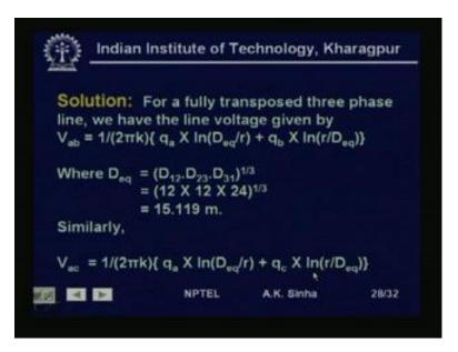
So, for solving this, we will take case of a fully transpose three phase line. So, we have the fully transpose three phase line. The voltage is given by the relationship V a b is equal to 1 by twice phi Epsilon, I am sorry, this is Epsilon into q a into log n D e q by r plus q b into log n r by D e q. Where D e q is equal to D 12 into D 23 into D 31 into the power 1 by 3. That is cube root of D 12, D 23 into D 31.
