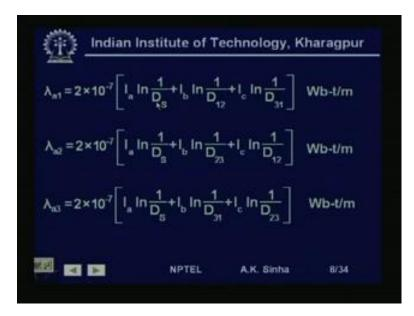
So, now, let us find out the flux linkage of phase a conductor in first one-third position of the conductor. This is, we write as lambda a 1, this is equal to 2 into 10 to power minus 7 into I a log n 1 by D s. Here, I am writing instead of r dash, because sometimes, we use, instead of one conductor more conductors. So, we are taking about the self distance, which is r dash for a single solid conductor line.
