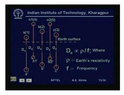
And are located directly below the overhead conductors, at a distance D e, as shown in this figure, that is here we have three phase conductors a, b and c. And we have two earth conductors are the ground conductors, which are n 1 and n 2. Now, what we he proposed as for such a system. He said that, the ground current flowing can be represented by conductors a dash, which is directly below a into the ground at a distance D, from that conductor.
