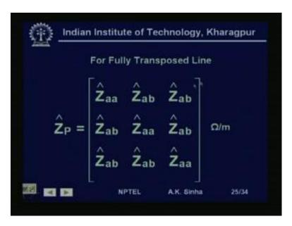
So, self impedance Z a a, will be same as Z b b, will be same as Z c c. That is all the three phase will have the same self impedances. And the mutual impedances will also be equal for all the three phases. So, Z a b and Z a c will be equal which will be also equal to Z b c and Z c a.
