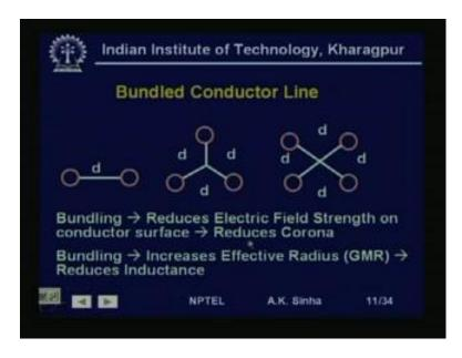
One is it reduces the electric field strength on conductor surface. And therefore, it reduces corona loses and radio interference and audible corona loses all the aspects which is associated with corona get reduced. Now, how does this happen. Now, if you see, if we use the conductor with the radius r, then it is volume will be phi r square. Now, if we take two conductors with the same, sorry, it is surface area is phi r square.
