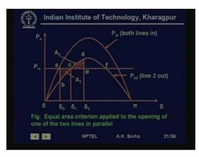
So, for a case, where we have a synchronous machine, supplying power to infinite bus bar, through two parallel transmission lines, we have the electrical power characteristics.
