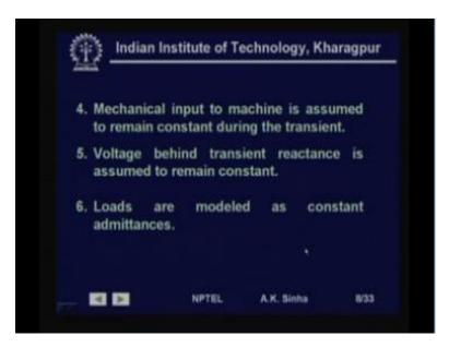
The fourth assumption, that we are making is mechanical input to the machine is assumed to remain constant, during the transient. That is the short period of study that we are doing. In that period, we assume that the speed governor system of the generator is not active enough to increase the mechanical input or decrease the mechanical input as required by the speed of the system.
