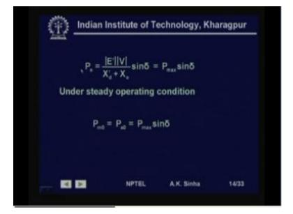
Now, P e the electrical output from this system will be given by E dash V by X d dash plus X e into sin delta. This is EV by X sin delta and total transfer reactance in this case is X d dash plus X e. So, this is, what we will get as the electrical output, which we call
