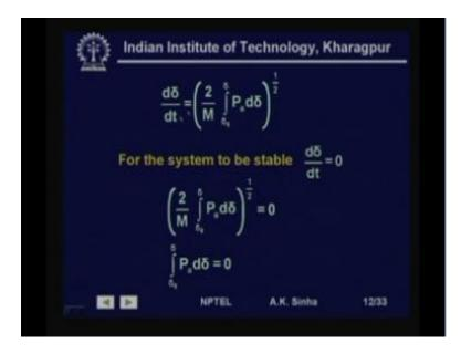
Now, from this, we can write d delta by d t is equal to 2 by M integral P a d delta from delta 0 to delta. That is limits to the power half that is square root of this. Since, this was square, so we remove this square, so we put a square root here. So, we have got this d delta by delta is equal to 2 by M integral this square root. Now, we have seen, that for the system to be stable, we must have d delta by d t is equal to 0 at some point.
