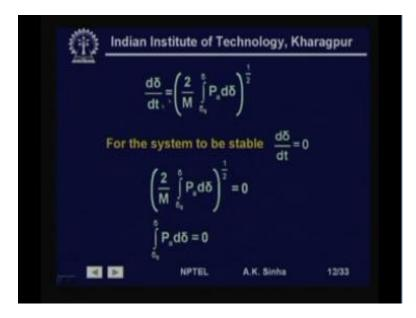
And if that happens, then what we have got is, basically this P a d delta integral is equal to 0, because A 1 plus A 2 is the total area, but A 2 is negative. So, A 1 minus A 2 is equal to 0 in this case. That is A 1 is equal to A 2, then we get this P a d delta integral is equal to 0. ((Refer Time: 51:40)). So, now, this is what we have seen that for the system to be stable. These two areas must be equal and that is why the name for this kind of analysis is equal area criterion.
