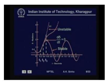
So, as we have seen that, when we make these assumptions, we have seen that. If we are working with ((Refer Time: 36:56)) the changing from P m o to P m 1. What we will find is, we are going to get an oscillation or a delta angle change, which will look like this. Here, I have model small damping, that is, if you see the oscillations are diagonal a little.
