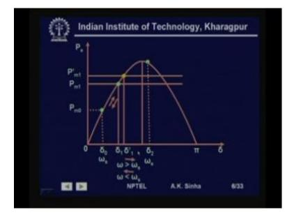
Now, let us see, how this whole dynamic process takes place. Let us say initially, we have the system, which is operating with the mechanical input P m 0 and electrical output as P e, which is equal to P m 0. And if P is equal to P m 0, then the power angle of the generator will be equal to delta 0. So, this is the initial operating point, the steady state point, which is there.
