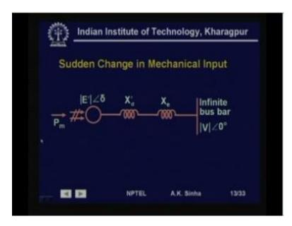
This let us see how we use for stability study. So, here we are talking about a sudden change in mechanical input the same thing which we discussed earlier. The machine internal voltage is E dash with an angle delta the X d dash is the machine transient reactance X e is the external reactance. And we have infinite bus bar, with a voltage V angle 0 degree; P m is the mechanical input to the system.
