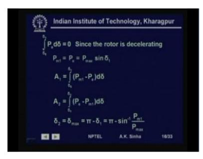
So, now, we have the integral from delta 0 to delta 2 of Pa d delta is equal to 0. Since the rotor accelerates in this part and decelerates in this part and reaches the synchronous speed at delta 2. So, we have P a d delta is equal to 0, that is P m 1 is equal to P e is equal to P max sin delta 1. This is delta 1. So, at this point b, we have delta 1 and P m 1 is equal to P e 1, which is P max sin delta 1.
