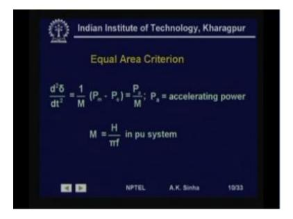
So, let us see what how we do that. We have the swing equation which we write as, M d 2, delta by d t 2 is equal to P m minus P e. I have taken this M from the left hand side to the right hand side. So, we write d 2, delta by d t 2 is equal to 1 by M P m minus P e, P m minus p e is the accelerating power. That is if the difference is positive, it is accelerating power, if the difference is negative, it is decelerating power.
