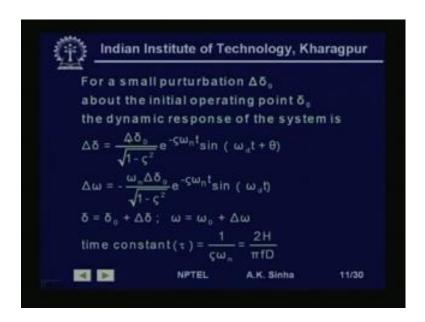
These can be obtained by looking at these relationship, delta, delta given by this relationship and delta omega is given by this relationship. So, we can plot delta with respect to time and for this particular system we have used delta, delta as 10 degrees. So, we have given a perturbation of 10 degrees and we have plotted delta and omega with respect to time. Then, we will get this, characteristics.
