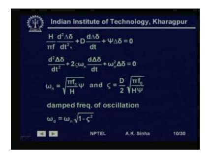
Let us go back to the small disturbances. So, writing the linearized swing equation M d 2 delta by d t 2 plus D, d delta by d t plus psi delta, delta. We are replacing M by H by pi f as we had seen earlier, that is writing instead of M. That is angular momentum, we are writing in terms of inertia, constant. Now, this expression can be written in a standard form like this.
