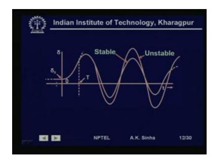
Then, we are saying the frequency of oscillation for this system is 1.345 hertz. This is a normal thing that we see, that is the damped frequency of oscillation for the dynamics of the system is normally of the order of 1 hertz or so. So, in this sense, that is why, when we are trying to analyze this system, we normally take a time period of a few seconds. Because, the frequency of oscillation is 1 hertz, so you get one cycle in one second or so.
