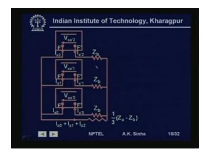
That is V a a 0 in which though the Z b is connected in series with this. So, I a dash 0 is flowing into this. So, this is V a a dash 0 minus Z b into I a 0 is the voltage across these two points. Similarly, V a a dash 1 minus Z b into I a 1 is the voltage, which is coming across these two points.
