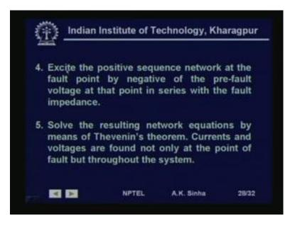
As what I said excite the positive sequence network at the fault point by negative of the pre-fault voltage at that point. In series with the fault impedance, this is what the Thevenin's theorem says that .We have reduced the network passive network by shorting all the voltage sources and replacing them by their appropriate impedances
