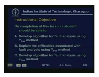
Well, the instructional objective for this lesson is that on completion of this lesson, you should be able to develop algorithm for fault analysis using Y bus methods. Explain the difficulties associated with fault analysis using Y bus method. Develop an algorithm for fault analysis using Z bus method.
