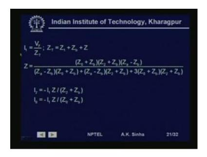
Now, as we said we can calculate the positive, negative and zero sequence current for this circuit. So, we can do that I 1 will be equal to V f by Z t that is if we see this circuit. V f is the voltage and this is the total impedance of the circuit is the Z t and we need to find out what is Z t.
