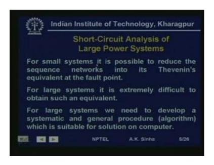
Well as we had discussed in lesson 29. That we can do symmetrical as well as asymmetrical fault analysis using Thevenin's theorem, but when we are trying to do it for a large system, trying to find out the Thevenin's equivalent of the network at the fault point as a very complex job.
