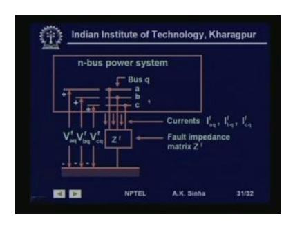
In which we have taken this bus q at which the fault has occurred the fault impedance is Z f and the a, b, c phase voltages are shown here for the bus q. So, with this we end today. In the next lesson we will talk about how to develop an algorithm for short circuit studies on large power systems.
