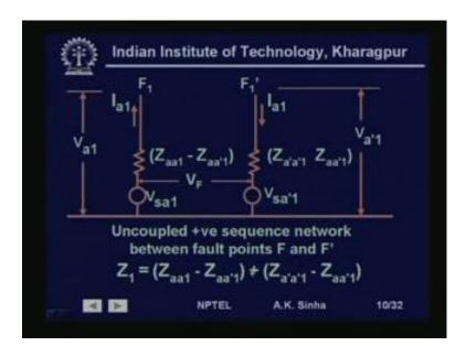
So, this is the relationship that we get which we can write in circuit form like this, where we have V s a 1 is the voltage of the internal voltages in the system. So, that is put here and we have the impedance Z a a 1 minus Z a a dash 1 as the series impedance connected to this source. And I a 1 is the current coming out at this point F 1. Similarly for the other side on the F dash side.
