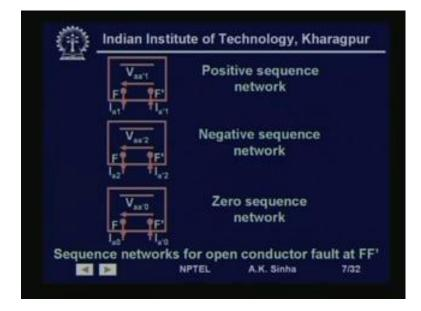
So and trying to obtain the sequence network for this we will also have these 2 points F and F dash. So, this is the reference there is the positive sequence network there is there is the reference. And we have F 1 F dash as the 2 points of indicating the fault. And voltage between these 2 points is v a a dash 1 which is the positive sequence voltage. And the current flowing is i a 1 and entering I a dash 1.
