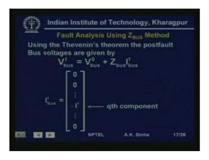
So, fault analysis using Z bus method. Now, again we have seen using the Thevenin's theorem the post-fault bus voltages can be returns as V bus as is equal to V bus 0 plus Z bus into I bus f. Now, what is this I bus f? I bus f is basically the current injections at various points when the fault as occurred.
