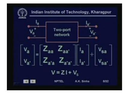
So, we need to take care of this using the theory from 2 port network. So, here I have shown this as a 2 port network, where we have I F flowing n on the input side. So, this side we have I a flowing n and V a is the voltage. And this side I a dash going out and V a dash is the voltage. Now, we can write down the voltage and current relationship for this 2 port network as V a V a dash is equal to Z a a Z a a dash Z a dash a and Z a dash a dash into I a I a dash.
