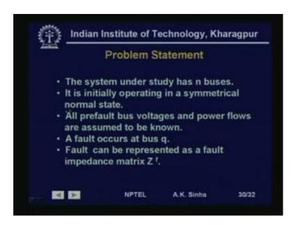
So, what we do is we say that the system under study has n buses, where n is very any number and large number normally. It is initially operating in a symmetrical normal state. That is what we assumed that initial conditions are steady state conditions all pre-fault bus voltages and power flows are assume to be known.
