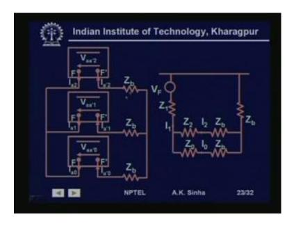
So, with this if you see then what happens if we go back to this circuit. What we find substituting Z a is equal to infinite means this becomes infinite. So, this is an open circuit, rest of the circuit, we do not have Z a. So, rest of the circuit remains as the case. So, this is what we get in this case that is this is the system, that we have, where we have Z a as here.
