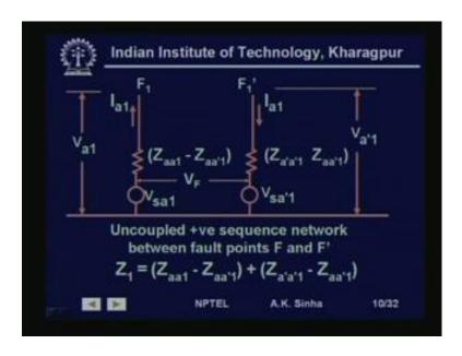
V f is equal to V s s V s a 1 minus V s a dash 1 this is what we have seen this is equal to V f. So, this is what we have. So, V f is this we have Z 1 Z 2 Z 0 ((Refer Time: 35:42)) that we have calculated earlier. So, these can be substituted here.
