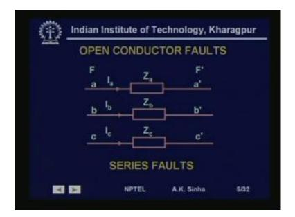
Now, how do we simulate these open circuit faults. Well, if you see here we have phase a, b and c in the 3 phases we have impedances Z a, Z b and Z c. Now, we are considering a fault occurs as between these points F and F dash on 2 sizes of these impedances. These impedances can be the line impedances themselves and the point F and F dash can be the 2 bus pass.
