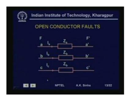
Now, for simulating the open conductor faults since we are simulating only 1 conductor or 2 conductor open faults. In case of 3 conductor open faults we do not need any analysis as such, because in that case there will be no current flowing through the system. System again will be symmetrical open circuit system.
