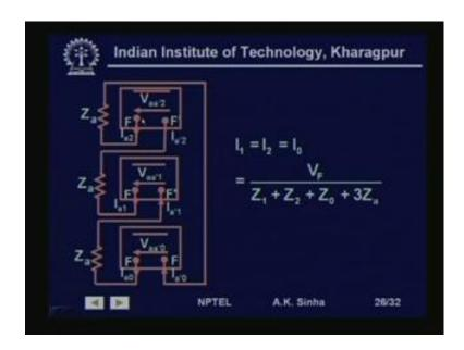
Here the, this is the zero sequence network Z a is connected in series like this. To F dash then from F again Z is connected to F here and then F dash here and then from F Z a connected and it comes to this point. So, the 3 networks are in series as such is Z a Z a and Z a connected here therefore, we get I 1 is equal to I 2 is equal to I 0. This is equal to V f divided by Z 1 plus Z 2 plus Z 0 plus 3 Z a.
