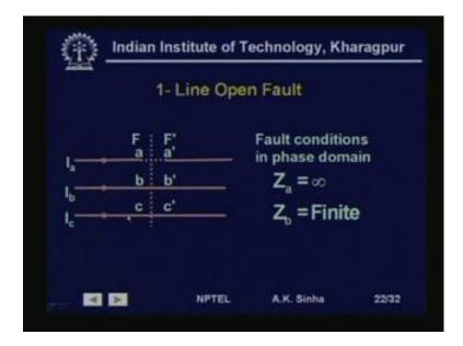
Now, we want to simulate 1 line open for a single phase open fault. Again here as we have seen we have this fault created between 2 points F and F dash. Now, in this case what we have Z a is infinite. If we see the previous system and Z b is finite. So, substituting Z b as finite. So, these 2 lines are connected and we have a finite impedance here infinite impedance here. There is a infinite impedance here because it is open here.
