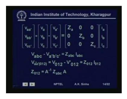
So, again we can write down the voltage equation for the system as V a a dash V b b dash and V c c dash in phase components. So, we this will be equal to V a minus V a dash V b minus V b dash V c minus V c dash, which will be equal to Z a into I a Z b into I b and Z c into I c.
