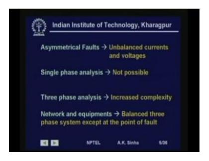
Now, we will talk about asymmetrical faults as we have said, a asymmetrical faults create unbalanced currents and voltages in the system. That is the three-phase symmetry of current and voltages are no longer maintained. Therefore the single phase analysis which we could do can no longer be used in this case, should we repeat them. Therefore, we need to do a three phase analysis in this case. Because, all the three-phase currents and voltages need to be found out.
