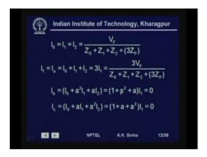
So, from this network if we need to find out the currents. The current I 0 is equal to I 1 is equal to I 2 will be equal to the voltage V f, here divided by all the impedances which are connected in series, so Z 1 plus Z 0 plus 3 Z f plus Z 2. Therefore we have here I 0 is equal to I 1 is equal to I 2 is equal to V f by Z 0 plus Z 1 plus Z 2 plus 3 Z f. And what is I f, I f is equal to I a, which is equal to I 0 plus I 1 plus I 2, which is same as 3 I 1.
