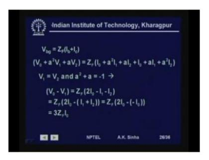
So, and V b is equal to Z f into I b plus I c. So, again substituting the values of V b we are writing plus Z f into I b plus I c. And then again taking help of V 1 is equal to V 2 and a square plus a is plus 1 is equal to 0 or a squared plus is equal to minus 1.
