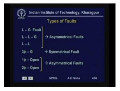
Well as we had discussed earlier about the types of faults the we have said the most common fault which occurs is line-to-ground fault. The next most common is line-toline-to-ground or double line-to-ground or line-to-line faults. These three faults which are much more common than the three-phase to ground faults are basically asymmetrical faults. Because, they create asymmetry in the current and voltage in the three-phases of the system.
