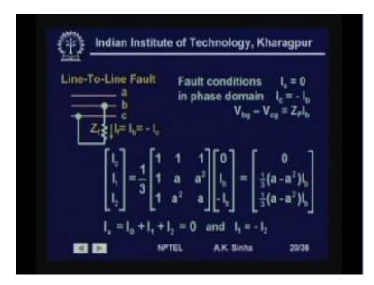
Now, let us take another kind of fault that is line to line fault. Now, for line to line fault we have the fault occurring at any bus, where between bus b phase b and c are faulted through an impedance Z f. So, now since we have assumed no pre fault currents which means I a is equal to 0. So, fault conditions in phase domain are I a is equal to 0, I b is flowing like this, I c is flowing like this. So, I b is equal to minus I c. So, I c is equal to minus I b.
