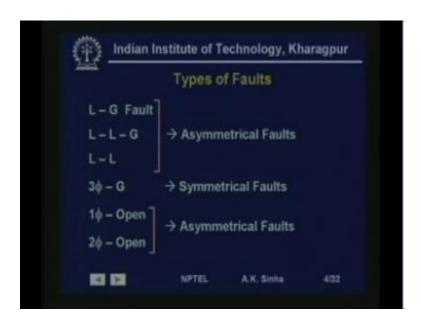
As we discussed in the previous lesson there are different kinds of faults which occur in power system such as line to ground fault or line to line to ground fault and line-to-line faults these are asymmetrical faults. Similarly, three phase to ground faults these are symmetrical faults. All these faults are basically short circuit faults.
