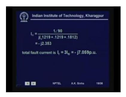
So, j 0.1219 plus j 0.1219 plus j 0.1812, so this comes out to be equal to j 2.353. So, this is the positive sequence current, this is same as the negative sequence current, this is same as the zero sequence current. The total fault current I f will be equal to 3 times I f 0 or I f 1. So, this is equal to j minus j 7.059 that is 3 times this value. So, what we see is 7 per unit current flows in the fault, when a single line to ground fault occurs at bus 3 of this system.
