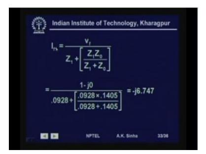
We can get the positive sequence current as if you see here this will be, this V f divided by the impedance this impedance plus these two impedances in parallel, So, that is what we have done Z 1 plus Z 1 Z 0 that is it should be Z 2 Z 0 Z 2 is same as Z 1. So, it is Z 2 Z 0 and Z 1 Z 0 divided by Z 1 plus Z 0. So, this is coming out to be equal to j minus j. 747
