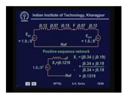
Now, first what we need to do is create the positive negative and zero sequence network for the system and find out the reduced network at the fault point. So, if we take the positive sequence network then we are assuming the normal voltage which is 1 per unit for the generator and same is for the motor.
