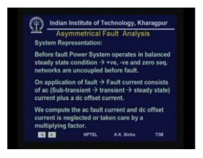
Now, in order to do the asymmetrical fault analysis, we need to make a system representation for which we make certain kind of assumptions. For the system representation, we assume that before fault system operates in balanced steady state condition. This is a valid assumption, because when the fault has not occurred as we have said earlier. The system operates as a balanced three phase system.
