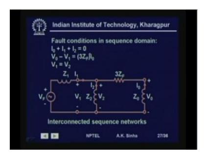
So, these are the conditions that we have got which tells us the sequence network connections are going to be like this. V 1 is this is the positive sequence network V f is the voltage source, Z 1 is the impedance and V 1 is the voltage between the fault point and the reference. We have the negative sequence network which is only having Z 2 no source. And the voltage across this is equal to V 2. So, V 1 is equal to V 2. So, this will be connected across this
