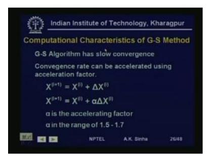
Now, computational characteristics of this method is very simple. But, it has slow convergence. So, for large power systems this method is generally not preferred. Now, people have tried to speed up the convergence characteristics of this by using some acceleration factor. So, instead of using this delta X, addition between the two voltages, we multiplied by alpha also. So, X at I plus 1th iteration is equal to X at i th iteration plus alpha delta X i.
