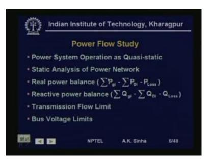
So, what we are trying do in power flow study. We are considering the power system operation as quasi-static operating condition. Power flow study is basically a static analysis of power network. We use the equations as real power balance at each bus. That is sum of the total generation, in the network is equal to the demand plus the losses. That sigma P g i minus P D i, this is the demand and minus P loss, the losses in the transmission system.
