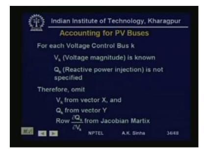
Now, what we do for P V busbars, for P Q busbars we have two equations. For P V busbars, we know the voltage magnitude. So, we do not need to write the equation for the voltage magnitude. So, what we do is, since Q is not known for that those busbars.
