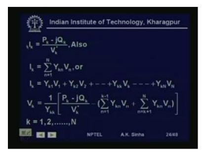
Now, I k is what, the current injection at bus I is equal to P k minus j Q k by V k conjugate. That is instead of writing, here S k is equal to plus j Q k, if you write P k minus j Q k. Then, we can write this as conjugate, V k conjugate into I k. And therefore, I k will be equal to P k minus j Q k by V k conjugate. So, this is what we have written here, I k is equal to P k minus j Q k by V k conjugate. And therefore, and we know I k is equal to this.
