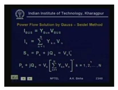
So, one of the techniques which is the simplest one is what we call the Gauss Seidel method. As we have seen earlier the power flow equations are non-linear. And therefore, we need iterative techniques for solution. Gauss Seidel is one of the those techniques, it is one of the simplest techniques for doing that. So, let us start with the very basics, we have the relationship I bus is equal to Y bus into V bus.
