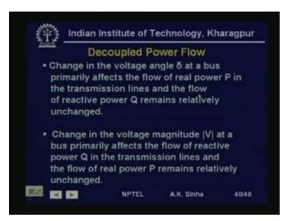
Now, one thing which we get is that, we know that the real power and voltage phase angle are very strongly coupled. And reactive power and voltage magnitude are strongly coupled. Whereas, there is a very weak coupling, between P and V, that is voltage magnitude and real power. And Q and delta, that is reactive power and voltage phase angle. This is also found from these, if we check the elements of these matrices.
