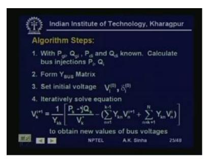
So, if we have this expression, now we can put it into an iterative solution procedure. The algorithm steps are with P g i, Q g i, P d i, Q d i known, calculate the bus injections P i, Q i. Form the Y bus matrix, set the initial voltages V i 0 and delta I 0. As I said earlier, we can choose for P V buses voltages specified, for all other buses very simple starting solution is, that the voltage magnitude is 1 per unit.
