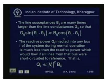
This is what we do in case of fast decoupled load flow algorithm. In fact, in that case the Jacobian matrix terms becomes constant. That is we have terms as V dash and V double dash which are nothing but the susceptance elements of the Y bus matrix. Negative of the susceptance elements of the Y bus, susceptance elements of the Y bus matrix.
