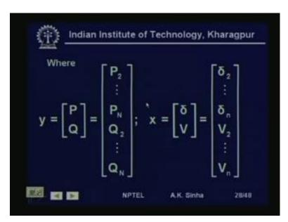
So, here y is equal to P and Q which is P 2 to P n and Q 2 to Q n. Now, here why we are not taking P 1 and Q 1, the reason behind that is, we have assumed that bus 1 is the slack bus. So, that is y we do not also calculate delta 1 and V 1. So, X is our delta V, which is delta 2 to delta n and V 2 to V n.
