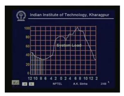
Well, as we can see from this diagram. The load on any system is not constant all the time, it keeps varying all the time. So, when we want to do a study, what we do is we take any time instant. And take the load at that time instant. In fact, what normally we do is, we take small time slices, in which we consider the load to be constant. And this we can keep the time slices every minute, or a couple of minutes.
