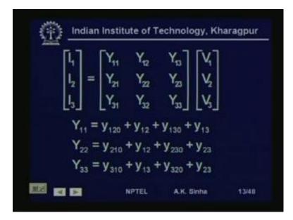
So, finally, we can write this as I is equal to this Y into V, where we as we said earlier the diagonal elements are nothing but sum of all the elements incident to that busbar.
