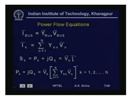
We can write the bus current injection at all the N buses in the system. As I bus is equal to Y bus into V bus. And where we have the current injection phasor at any bus k, is written as I k is equal to summation n is equal to 1 to capital N, where capital N is the number buses is equal to Y k n into V n, where Y k n is a complex admittance of. That is the k, k through and nth column element of the Y bus matrix. And V n is the voltage phasor at bus n.
