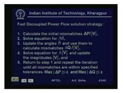
So, again the algorithm for fast decoupled is shown here, which is what we have done earlier.
