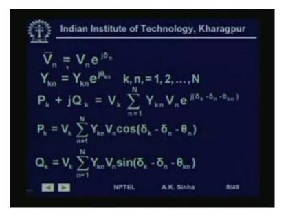
Where the voltage phasor at bus n, any bus n is V n is equal voltage magnitude at that bus, this V n e to the power j delta n, where delta n is representing the phase angle of the voltage phasor. Y k n is equal to, since Y k n is a complex quantity. This again in phasor form can be written as Y k n e to the power j theta k n, where k n n are from 1 to N. So, now in these terms, if we want to write this in terms of phase angles and magnitude for the voltage and the admittances.
