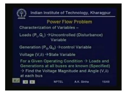
Now, we will go into the power flow problem itself. Now, let us see what we have. Now, we have loads P L and Q L, which are uncontrolled or disturbance variables. Because, loads are not controlled by us, it is controlled by the consumers. So, the power system operator has no control on the consumers. They can switch on or switch off their loads, as they feel like. So, these are controlled or disturbance variables.
