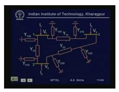
So, if we do that then for each line we have a nominal pi model associated with it. Where these elements Y 2 3 0 and Y 3 2 0 are basically the half line charging susceptances, associated with the line 2, 3, a same thing for the other lines. Here, what I have done is instead of writing the injections P 1 Q 1 and P 2 Q 2, P 3 Q 3, we have converted them as currents for the time being. So, we have a current injection I 1. We have a current injection I 2 here, and a current injection I 3 here.
