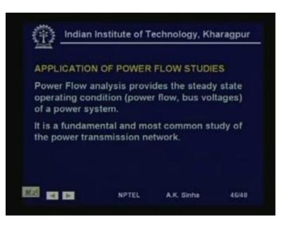
Now, what are the applications of the power flow analysis. Power flow analysis provides the steady state operating condition. That is power flow bus voltages in a power system. And it is a fundamental and most common study of power transmission network. (Refer Slide Time: 57:55)
