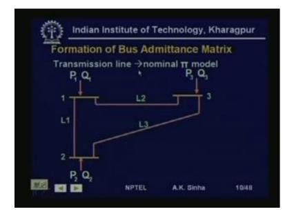
Now, let us take a small system to show, how we can find out the Y bus elements for the system. Now, this is a simple 3 bus system, where we have power injections P 1 Q 1 at bus 1, P 2 Q 2 at bus 2, P 3 Q 3 at bus 3. And we have line L 1 connecting bus 1, 2, L 2 connecting bus 1, 3 and L 3 connecting bus 2, 3. Now, for this system these transmission lines as we have seen earlier are modeled as nominal pi model.
