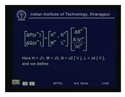
Now, we can try and make some improvement in this. That is the calculation of Jacobian elements can be again reduced. If we multiply the element of this, del P by del V term by
