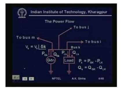
Now, if we look at a single bus here, which has a generation said we are taken a bus k, it has a generation P G k, and reactive power generation Q G k. And this bus has a voltage V k, which we write as V k magnitude and angle delta k. So, this is a complex voltage, which has a magnitude and a phasor angle delta. Now, this bus also has a load P L k and a reactive power load Q L k. So, real power P L k and reactive power Q L k are the loads at this bus.
