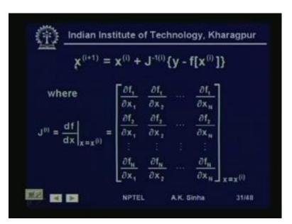
So, once we have this expression like this, in iterative form. We can write that x at I plus 1th iteration is nothing but equal to x at i th iteration. Plus J inverse calculated at i th iteration value, that is at x is equal x at i th iteration into y minus f at calculated for x at i th iteration. And this J is the Jacobian matrix, because we have n number of equations. And this is the partial derivative of all those equations.
