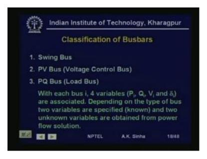
Now, what about other busbars, now some of the busbars where both P and Q are known. Mostly these are the busbars, where the loads are there. So, load buses are substations, which are connected to supply consumers loads. So, there we know the real and reactive power, supplied to the consumers. So, those buses are called P Q busbars or load buses.
