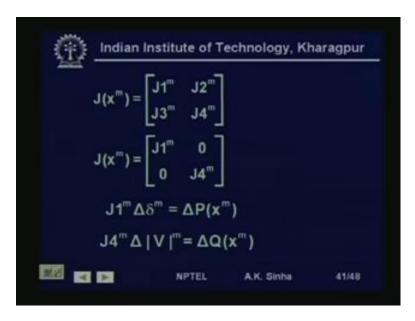
So, this is what we try to do, that is here as it is shown these two sub-matrices are assumed to be 0. If we do that, then we have two separate equations, that we can solve and the size of the Jacobian matrix becomes much smaller. This is what we do in decoupling.
