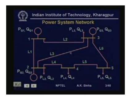
Now, let us take a very simple example of a power system network. Now, here this network, we have 5 nodes, 1, 2, 3, 4 and 5. Some of the nodes, we have generators associated with it. Like node 1 has a generator, node 2 has a generator, node 3 has a generator. Some of these nodes have loads on them, like node 2, node 3 has a load. Node 2 also has a load, node 4 has load, a node 5 also has load here.
