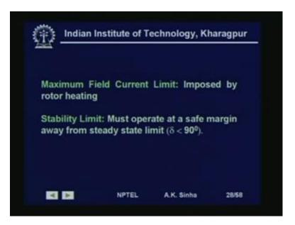
Maximum field current limit. Again we cannot excite the machine, beyond a certain value. Because, the rotor current is going to exceed and rotor heating is going to go on. Therefore, the maximum current that can be allowed in the rotor limits, the reactive power supply also. Stability limit, this is basically a dynamic aspect. That is generally we cannot allow this machine to work beyond a delta angle of 90 degrees.
