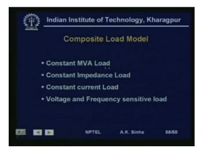
So, we can composite loads, can be modeled as constant MVA load. Constant impedance load, constant current type loads and voltage and frequency sensitive loads. All these types of load can be aggregated as a complex model.
