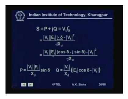
So, now if we substitute that, that is V t into I a conjugate. Then we are going to get this relationship. And if we substitute for all these delta angle here. Then we get finally, P is equal to V t into E i by X d into sin delta. And Q is equal to V t by X d into E i cos delta minus V t. Now, these are very important relationships. It tells us that, the real power output of the synchronous machine depends on the power angle delta.
