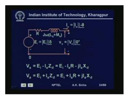
So, this is what we get. And the circuit model for the synchronous machine, can be put like this; where this for the machine acting as a generator. We have V a is equal to E a or E i minus R I into R plus j omega L s plus M s. That is E i minus I a into Z d, which is equal to E i minus I a R minus j X d into I a. If it is acting as a motor, then we are exciting from here.
