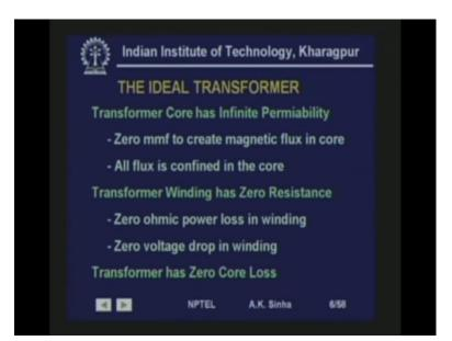
Now, this transformer we assume has infinite core permeability. That is the permeability of the core is infinite, what does it really mean? It means that, there is no mmf required to create the magnetic flux in the core. That is there is no current, which is exciting current required to create the flux. All flux is confined in the core. That is it again says that, the core since it has infinite permeability all the flux will try to reside inside the core.
