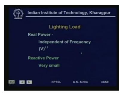
We have already discussed about the characteristics of these. Like lighting load has a real power independent of frequency and voltage to the power 1.5 reactive power is very small.
