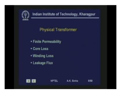
Now, in case of a physical transformer, what we have a finite permeability. There are core losses, there is loss in winding. Because, winding has a resistance and there is going to be voltage drop. Because, again the core does not have a infinite permeability. So, some flux will pass through air path.
