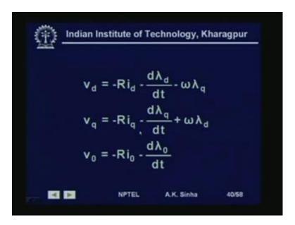
So, we do that, then we will write all the relations for voltage, and the flux linkages. In terms of D Q 0 frame of reference. And we avoid the time varying inductances in this case.
