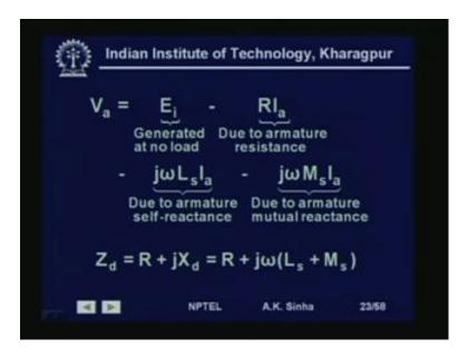
Terminal voltage is going to be equal to the generated voltage minus what? The drop, voltage drop due to current flowing through the armature winding resistance. So, due to armature resistance, the voltage drop R I a, minus again the drop due to the self reactance of the rotor winding. Since, the winding well is wound as a coil, so it has a reactance. So, self reactance or self inductance L S. So, it is j omega L s into I a, this is a drop due to armature self reactance.
