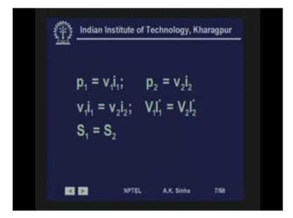
So, what we find for a ideal transformer, the input power is equal to the output power. What we have as the input power, the instantaneous value of the input power, that is p 1 is equal to v 1 into i 1. Now, these small case letters are meant for instantaneous values. So, the instantaneous power at the input end is v i into i i. And similarly, p 2 is equal to v 2 into i 2.
