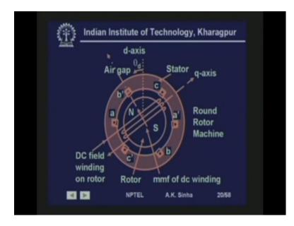
Now, again for synchronous machines also we have. Normally two kinds of machines based on the type of the rotor of the machine. One model that we use as shown, here where we have the rotor which is around cylindrical structure on which the winding is placed. These kinds of machine are called round rotor machines. And these are generally used for large turbo alternators, which are run by steam turbines.
