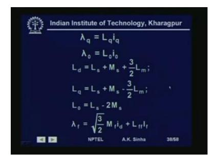
Then we can write all these equations for inductances, and the flux linkages. And we find that in this case most of the inductances are have become constant, because now the D Q 0 frame is also rotating along with the rotor. So, these time varying inductances are no longer there.
