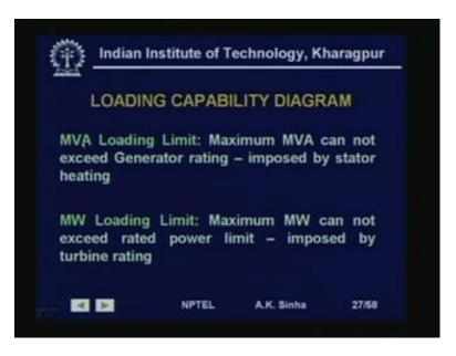
Now, how much we can load the machine, a synchronous machine can be loaded up to what extent. This we can find out by looking, at what are the limits which come into play. First is MVA loading limit, the maximum MVA cannot exceed the generator rating. Why, that simply depends on the maximum current that can be allowed, because if we allow more current than the rated value, the heating is going to be much more than the cooling which is provided.
