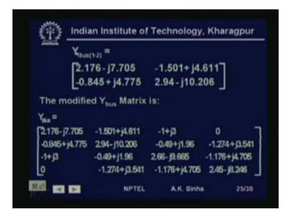
So, if we do that we will get Y bus 1 2 as like this. And so these four elements of Y bus gets replaced, by these elements. Then final Y bus comes out to be like this. So, this is how we can take here of the regulating transformer in power system. So, we can have either off nominal turns ratio. Or that is the off nominal tape position of the transformers for voltage control.
