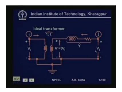
Because, if we recall our early lesson on per unit system. If we have a nominal, that is if we have the tap position at the nominal. Then the voltage ratio on the two sides is same
