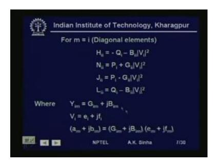
Similarly, the diagonal elements can also be computed as shown here as H i i is equal to minus Q i minus B i i V i magnitude square. N i i is equal to P i plus G i i V i square and this should be L i i is equal to P i minus G i i V i square, this is M. And this is L i i is equal to Q i minus B i i V i square, where Y i m that is the i m th element of the admittance matrix is written as G i m plus j B i m.
