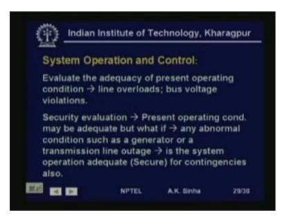
Now, for system operation and control, how we can use this. Again evaluate the adequacy of the present operating condition. That is the present operating condition all the flows and voltages are within limits. Like this is what any line overloading is there or not bus voltage volitions are there or not, we can check these. Of course, most of time we will find no such thing for a normal system should be there.
