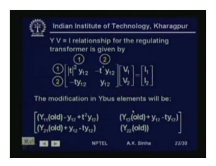
So, if you do that, then Y V is equal to I relation for the regulating transformer as given by this relationship. And therefore, the modification in Y bus elements will be what? See we had, we are going to have modification where y 1 1, y 1 2, y 2 1 and y 2 2. These are the four elements in the Y bus, which will get modified. Because, we are say that we are having a regulating transformer with the turns ratio of 1.05.
