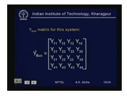
We can get the admittance for each line, that is we can find out the Y i j for each line. That will be simply 1 by R plus J x term. So, we can find that out, what we will finally get is the Y bus matrix which will be a 4 by 4 matrix for this system.
