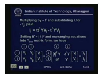
So, multiplying by minus t conjugate and substituting for I i. That is for minus t conjugate I j will yield I i is equal to t t conjugate into Y into V i minus t conjugate Y into V j. So, this is what we will get, that is we have multiplied the equation by t conjugate. And we are writing minus t conjugate i j is equal to I i. And therefore, we will
