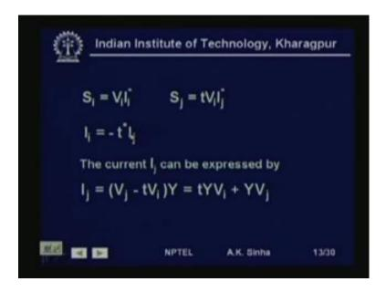
Now, the complex power S i is equal to V i I i conjugate. And complex power S j is equal to t V i into I j. That is if we see here t V i is the voltage and if I j is the current flowing in this direction. Then, the complex power entering from this side is S j and that
