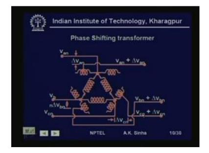
Similarly, instead of having a voltage control, if you want to have a control over the power flow on the transmission line. Then what do we need, we have already seen that the real power flow on the transmission line is dependent on the phase angle at the two ends of the line. That is it is dependent on delta i minus delta j. Now, if you want to increase the power flow and this line from i to j, then delta i minus delta a j must be increased.
