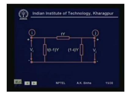
Then from this we can form a pi equivalent circuit for the regulating transform. But, this is not feasible for the phase shifting transformer, where t is a complex quantity. In that case, this will not be possible to do by the physical elements. Because, you are going to get terms, which will require negative resistance and so on. Therefore, we do not form a pi equivalent circuit for the regulating transformers, when we are using phase shifting transformers.
