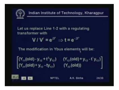
Now, let us instead of the voltage control. If you want power flow control, then we use phase angle, shifting. And let us say we have V by V dash is equal to 3 degrees. So, here we are not trying to change the magnitude of the voltage, we are only trying to give a phase shift of 3 degrees. So, it is e to the power j 3. Now, this will give again t is equal to 1 by this, which is same as e to the power minus j 3 degrees.
