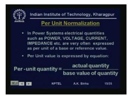
So, in power system electrical quantities such as power, voltage, current, impedance etcetera, are very often expressed as per unit of a base or reference value. That is what we do is we represent these values on a reference, with respect to a reference or a base value, per unit value is expressed by the equation. Per unit quantity is equal to actual quantity divided by the base value of that quantity.
