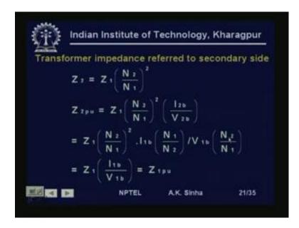
And if it is referred to the other side, secondary side, then Z 2 is equal to Z 1 in to N 2 by N 1 square. Therefore, Z 2 per unit will be equal to Z 1 into N 2 by N 1 square which is nothing but, Z 2 into I 2 base by V 2 base, this well again substituting the values we have Z 1 in to N 2 by N 1 square into I 1 base into N 1 by N 2. For I 2 base we can write and divide by V 2 base can be written as V 1 base into N 2 by N 1.
