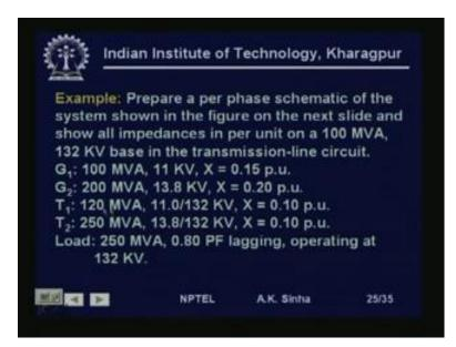
Now, let us take a simple example for this per unit representation. Here we have taken a problem where we say that prepare, a per phase schematic of the system shown in the figure, which is shown in the next slide. On the next slide, and show all the impedances in per unit on a 100 MVA base. 132 KV voltage base in the transmission line of the circuit. That is the impedance the power base for the whole system is chosen as 100 MVA.
