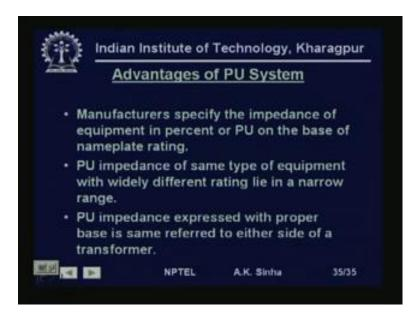
Now, we will see what are the advantages? After we have solved this problem. We will can see what are the advantages of this per unit system? One is manufacturers specify the impedance of equipment, in percent or per unit on the base of the nameplate rating. That is what we were given is for a generator at 100 MVA base and it is rated KV the reactance was given. Similarly, for generator G 2 at 200 MVA and it is rated voltage the reactance was given.
