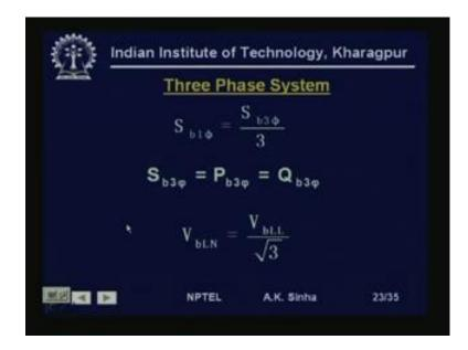
Till now we talked about single phase system. The per unit system representation can be extended. Or used in 3 phase system also in a similar way. What we have is for a single phase system, if we have chosen a base S base for single phase, this is equal to S base for 3 phase system divided by 3. We know that for any equipment rating. If we have the 3 phase rating, then per phase rating is going to be 1 3rd of that.
