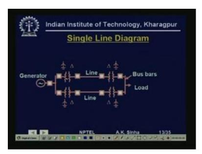
Now, here for an example, I am showing you a single line diagram of a power system. Now, in this diagram, you see we have a generator, we have circuit breakers. Then we have a bus-bar which is connecting this generator to various transformers. We have transformers connected to the bus-bar through circuit breakers. We have another transformer here for the other line. And the lines the two parallel lines are connected to the transformers through circuit breakers shown here.
