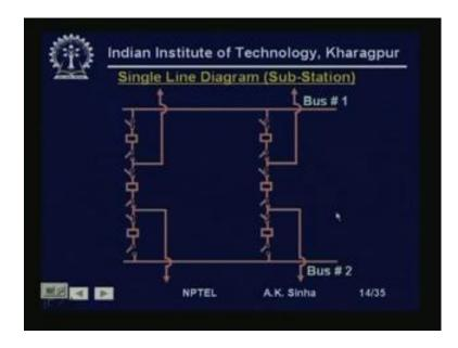
Next we have a substation with 2 bus-bars and 4 transmission lines. We have these transmission line 1, 2, 3 and 4 connected to these two bus-bars. By means of circuit breakers shown here, and the isolator switches shown here. So, this is how we represent a power system network, using single line diagram. This is much simpler, much easier to understand, because it is showing you the relative interconnection of the various components. And it is much more simplified and easy to see and draw.
