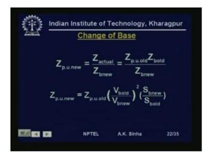
In power system, we also use equipments at various with various ratings, different ratings. And therefore, we need to convert the impedance values from one rating to another. Because as I said earlier the equipment manufacturers will generally specify the value of the impedance of any equipment, in terms of percentage, or per unit values based on the name plate rating of that equipment.
