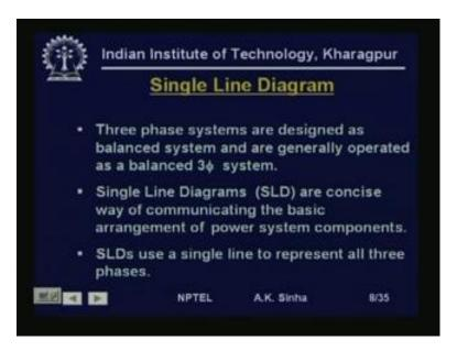
We know that 3 phase systems are designed as balance system. And are generally operated as a balanced 3 phase system, which means that all the equipment which are the 3 phase equipment like generators, motors, transformers. All are designed to be balanced system means. All the 3 phases have equal impedances have the same voltage levels and so on.
