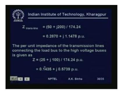
Therefore, we can find out for each transmission line, the per unit value of the impedance. So, for the transmission line having impedance 50 plus j 200, the per unit value comes out to be 0.2870 plus j 1.1478 per unit. Similarly, for the transmission line having impedance value of 25 plus j 10, the value comes out to be 0.1435 plus j 0.5739 per unit.
