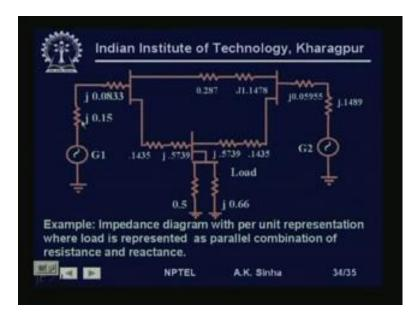
And therefore, if we put all these impedance values on the single line diagram. Then we get this network diagram. The generator with its impedance at j is equal to 0.15 generator G 1. Then we have the transformer impedance, then we have the transmission line
