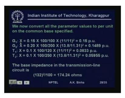
Now, we convert all the parameter values to per unit on the common base specified. So, G 1 the value given is X is equal to 0.15. Now, we are converting it to our new base. So, S base old by S base new is both are 100. Similarly, the voltage also base old and base new voltage are also same. So, the value of the impedance remains same. So, using the same relationship, we find out the value of reactance for G 2 which comes out to be 0.1489 instead of 0.2
