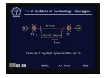
So, this is our system we have a generator G 1, connected through a transformer T 1 to this bus. And a generator G 2, connected through transformer T 2 through this bus. This is, these two transformers are step up transformers. And we have three transmission lines, working at 132 KV and a load of 200 MVA at 0.8 power factor lagging connected at this bus. Now, let us see how we convert this in per unit system. The impedance values, here for the transmission lines are given in ohms.
