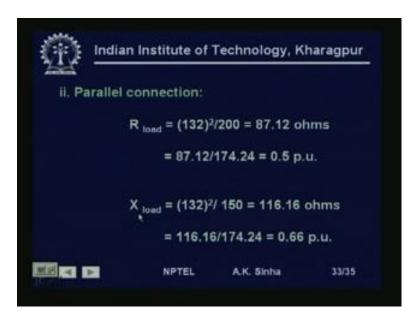
If we take the parallel combination, again we can find out the value of resistance part, which is KV square divided by P. That comes out to be 87.12 ohms which in per unit comes out to be 0.5 per unit. The reactive part can also be found in the same way V square by Q, which is coming out to be 116.16 ohms which comes out to be 0.66 unit.
