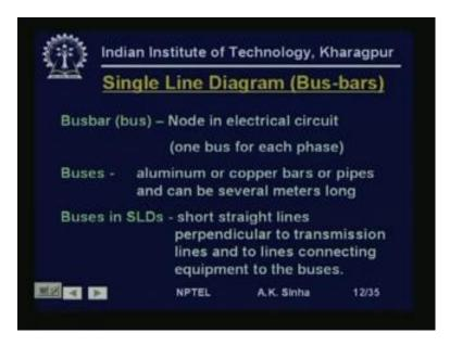
Now, in power system we have a concept of a bus-bar. Bus-bars are nothing but, nodes in electrical circuit. So, basically in power system, we call these nodes of electrical circuit as the bus-bars. This is required in power system, because you cannot join various lines, which may be very thick lines just by connecting at one point. So, what is used is a long bar is used. And these various lines and components are connected to this bar by means of nuts and bolts.
