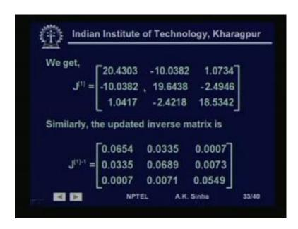
Another accept, which is very important here is that the Jacobian matrix. That we have here, since it is a three bus system and all the buses are connected to all other buses is a full matrix. But, in a general the Jacobian matrix, will be a spars matrix. Just like, the Y bus matrix, which is a spars matrix. Because, we know all the buses are not connected to all other buses in a large system.
