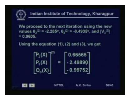
Now, again using these values, we can compute the calculated values for P 2, P 3 and Q 3, which comes out to be this much. That is P 2 with the new values of the voltage magnitude and angle comes out to be 0.66565. And the P 3 comes out to be minus 2.49890 and Q 3 comes out to be minus 0.99752.
