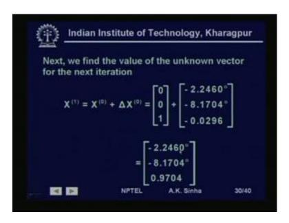
So, using this error values at the first iteration, we get the updated value of the state variables at the first iteration as X 1 is equal to X 0 plus delta X 0. So, the initial guess value of X 0 was 0 degree 0 degrees and 1 per unit. So, we add to this the delta X, which is the value, when we substitute. So, we get the value of the state variable, after first iteration as minus theta 2 is equal minus 2.246 degrees. Theta 3 is minus 8.1704 degrees and V 3 as 0 0.9704 per unit.
