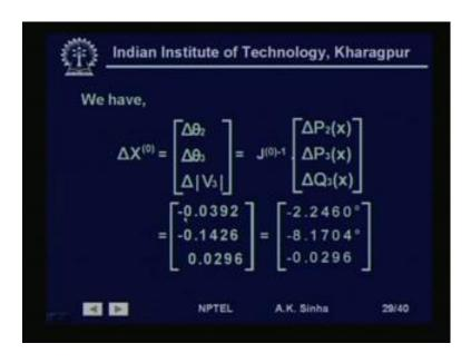
So, using that, we can calculate the change in the state vector. So, initial error of the state vector, will be given by J, 0 inverses in to del P 2, that is del Y. So, if we substitute that then we solving it, we will get the value of delta X, 0 as 0 minus 0.0392 minus 0.1246. So, this is delta theta 2, this is delta theta 3 and this is delta V 3. So, these values, you mind it, the angle values, when we calculate, using this will be in radians.
