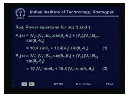
Now, substituting, so real power equations for bus 2 and 3, we can be written in this form. Because, here we have seen that the real part for the Y bus is 0. So, G's are not there. So, only B is present. So, we write the equation like this V 2, V 1, B 21 sin theta 2 minus theta 1 plus V 2, V 3 into V 23 sin theta 2 minus theta 3.
