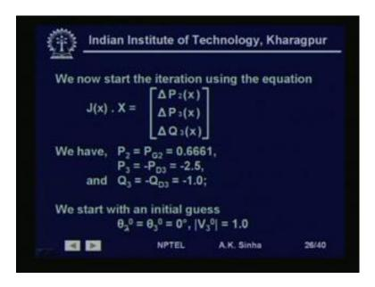
Now, we can start the iteration using the equations J, X J, which is a function of x into X is equal to Y, which is delta P 2, delta P 3 and delta Q 3. Now, we have the specified value of P 2, which is P G 2 is 0.661, 6661 per unit. P 3 the injection is minus P D 3, this is equal to minus 2.5 and Q 3 is equal to minus Q D 3, which is equal to minus 1.0. Now, if we said earlier, we start with an initial guess for the unknown voltages magnitude and
