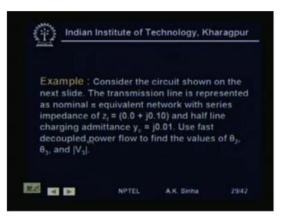
So, consider the circuit shown on the next slide, the transmission line is represented as nominal pi equivalent network, with series impedance Z l is equal to 0.0 plus j, 0.1 and half line charging admittance Y c is equal to j 0.1, 0.01. Using fast decoupled power flow, find the values of theta 2, theta 3 and V 3.
