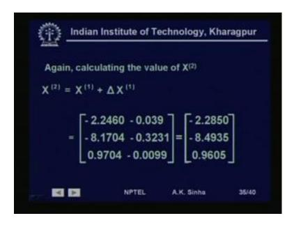
So, again, we can get the updated value at the second iteration as the value at the first iteration plus the change or the error computed after first iteration. So, when we do that, we get the values as minus 2.2850 degrees minus 8.4935 degrees and the voltage magnitude V 3 as 0.9605 per unit.
