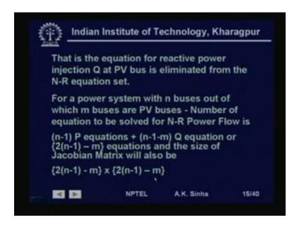
That is the equation for reactive power injection Q at P V bus is eliminated from the Newton Raphson equation set. Therefore, we find that for a power system with n buses, n buses out of which m buses are P V buses. What is the number of equations to be solved for Newton Raphson power flow? Well, as we have seen we need to write n minus 1 P equations. Because, for n minus 1 bus, except for the slack bus, the real power injection at all other buses are specified.
