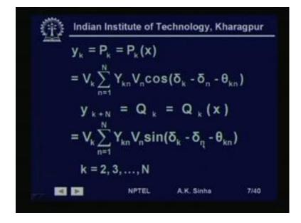
So, for any particular bus, we can write the equation y k is equal to P k, which is P k a function of x. In this term and we can arrange all the reactive power injections from k plus N to k plus. This will be equal to 2 N basically. So, k is equal 2 to N will be the first
