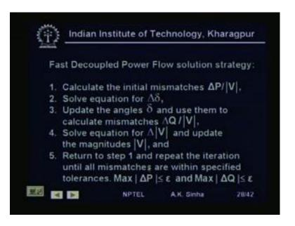
Now, we will take one example, for solving a power flow using fast decoupled method.
