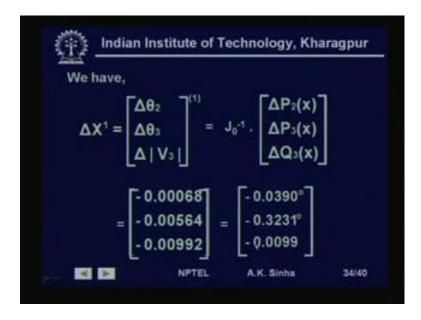
And once, we have this, we can get delta X 1, the error in state variables at first, after first iteration. So, this comes out to be 0.00068. That is delta theta 2. After, first iteration comes out to be this, delta theta 3. After, first iteration comes out to be minus 0.00564. Radians and delta V 3, after first iteration substituting the first iteration values or solving after using the first iteration values, comes out to be minus 0.00992.
