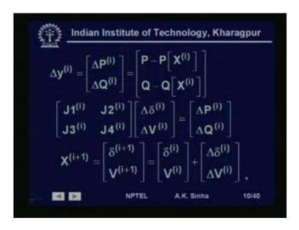
For power flow term, we can write delta y i is equal to delta P i and delta Q i. That is the change in real power and change in reactive power at ith iteration. This will be nothing but equal to the P value, which is specified at the buses minus P value, which is calculated with the state variable x are V and delta calculated at ith iteration. Same thing for Q, Q is specified value at that bus minus Q calculated with x at ith iteration.
