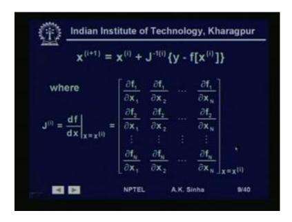
In and in a iterative term, the Newton Raphson power flow equations can be written in terms of x. At iteration i plus 1 is equal to x at iteration i plus J inverse at iteration i into Y minus f x calculated at the x values at ith iteration. So, with this as an iterative form is the basic Newton Raphson algorithm. That we have for power flow solution, where J is basically the Jacobian matrix d f by d x at x is equal to x i.
