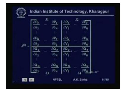
Now, as I said earlier, the Jacobian matrix, we have divided into four parts. J 1, J 2, J 3, J 4, where J 1 is del P by del delta, sub matrix J 2 is del P by del V sub matrix. And J 3 is del Q by del delta sub matrix and J 4 is del Q by del V sub matrix. So, this matrix as we are seeing is N minus 1 into N minus 1 for J 1 and similarly for J 2, J 3 and J 4. All these matrixes are N minus 1 to N minus 1, total size of the Jacobian is 2 into N minus 1.
