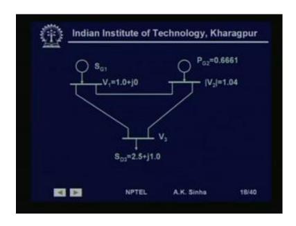
Here, we have a three bus system, this is bus 1, this is bus 2 and this is bus 3. Now, bus 1, we have chosen as a slack bus. So, here the voltage magnitude, as well as angle specified. We have port here voltage magnitude as 1 per unit and angle is 0 degrees. That is, in rectangular coordinate form, we can write it as 1.0 plus J 0. So, voltage magnitude and angle at this is specified. The real and reactive power injection at this bus is unknown.
