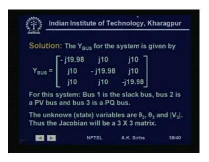
Now, first thing, what we will do is, we will form the Y bus matrix for the system. Now, as we have seen the real power, the series reactance for the line is 0.1. So, in terms of admittance, we will get this as minus 10. So, and the off diagonal terms for the admittance matrix as we have seen is minus Y i j. So, we have got J 10, J 10 as for all the lines are having the same impedance. So, we have got this.
