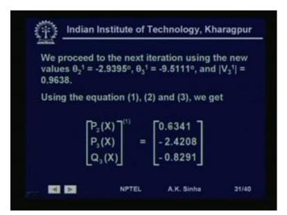
So, once, we have these values now. So, using we proceed to the next iteration using the new values. So, when we substitute this value, again we will calculate P 2, P 3, Q 3 at the first iteration, which we get like this.
