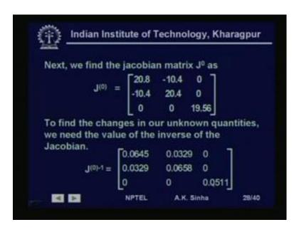
Similarly, we can calculate the Jacobian matrix elements by substituting the value of the state variables with the initial the guess values. So, this comes out to be the 3 by 3 Jacobian matrix, 20.8 minus 10.4, 0 minus 10.4, 20.4, 0, 0,0 19.56. So, this is 3 by 3 Jacobian matrix, that we have. So, what we need to do is, we can solve the equation now, that del P del Q is equal to J del X or that is del delta del V.
