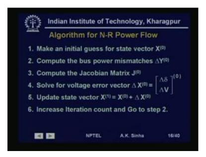
So, what is the algorithm for Newton Raphson power flow? What we have to do is, first we will make an initial guess for the state vector X 0, as we have said earlier the easiest guess, that we have is, a flat voltage start. So, for all the buses, except the slack bus and P V buses, we choose the voltage magnitude, as 1 per unit. And for all the buses, except the slack bus, we have the voltage angle initial guess as 0 degrees.
