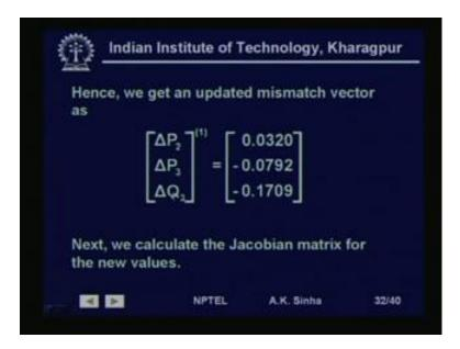
So, we can calculate delta P 2 delta P 3 and delta Q 3, which will be again calculated value specified value minus the calculated value, where the calculated value is computed using the updated or the first iteration value of the state variables. So, when we do that, we get these values like this. Now, we calculate the Jacobian matrix with the new values of X.
