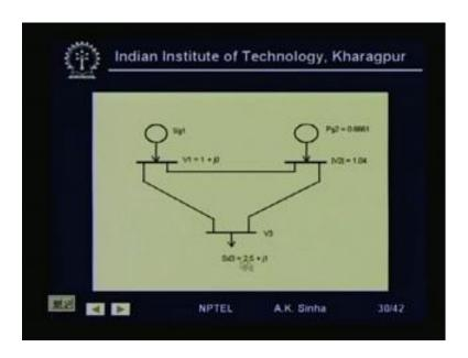
Now, if we see this system, this is a three bus system. This bus 1 is a slack bus, where the voltage is specified as one angle 0. That is 1 plus j 0, bus 2 is a P V bus, where we have the real power injection given as 0.6661 per unit and the voltage magnitude at this bus is given as 1.04 per unit. Bus 3 is a P Q bus, where the load value is given as 2.5 plus j 1.
