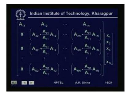
We will see, how we do that? That is, we can multiply this by row by A 21 by A 11. So, we multiply this row by A 21 by A 11 and then subtract from the second row. Then, we will get this as A 21 minus A 21, so this becomes 0. This element will be A 22 minus A 21 by A 11, which is this all the elements of the this row, has been multiplied by that into A 12 will be the element of this row.
