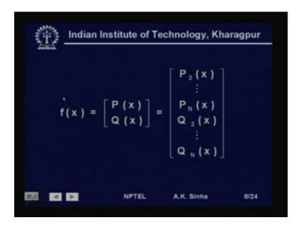
Therfore, we can write f x is equal to to P x, Q x. where, the P x, Q x of this vector f x is P 2 a function of x upto P N. All these are function of x, Q 2 to Q N; all these are also funciton of x, where x is basically the voltage. Angle delta and the voltage magnitude V, at all the buses.
