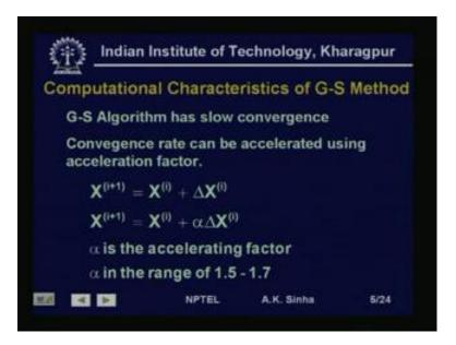
Now, we will talk about computational characteristics of Gauss Sidel mehtod. Gauss Siedel algorithm has one problem, that it is convergence is somewhat slow. In the sense that, suppose if you have a very large system. Suppose, you are having a system with more than 100 buses or a 100 bus system, let us take for example. Then, the number of itertaions, which one needs to solve these node flow equations for hunderd buses.
