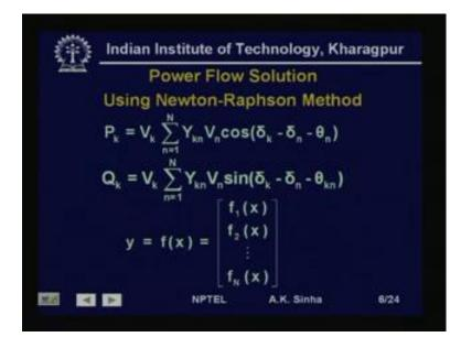
So, we will see, how we apply newton Raphson method to power flow analysis. Now, here, as we had seen, if we write the power flow equation for each bus in terms of power injections, real power injection and reactive power injection, seperately. Then, we get real power injection P k is equal to V k summation, Y k n, V n cos, delta k, minus delta n, minus theta k n, for n is equal to 1 to capital N.
