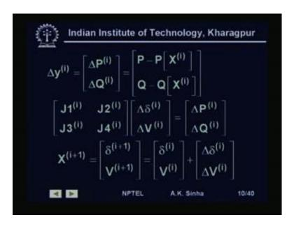
We can find out the mismatch using this relationship P specified minus P calculated with the value of x known at the initial guess, Q specified minus Q calculated, with x at the specified value. So, using this, we can find out this delta P and delta Q, which is basically our delta y. So, compute the bus power mismatches delta y, next step is compute the Jacobian matrix J 0. That is with the initial guess state vector x.
