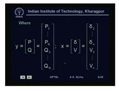
Where, y is basically a vector of real power injections P and reactive power injections Q. Here, we have assumed that bus 1 is a slack bus for our purpose. So, for slack bus since we know the voltage magnitude an angle, we do not have any real power or reactive power specified. So, we do not have any P 1 and Q 1 in this vector of y. So, we have P 2 to P N and Q 2 to Q N.
