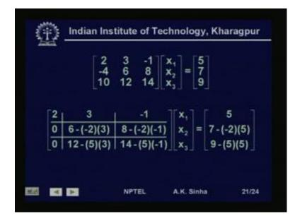
So, let us take a small example. Here, we have a 3 by 3 matrix, our A matrix is a 3 by 3 matrix. The first row is having 2, 3 minus 1, that is the equation, that we have is 2 X 1 plus 3 X 2 minus X 3 is equal to 5. The second equation we have is, minus 4 X 1 plus 6 X 2 plus 8 X 3 is equal to 7. The third equation is 10 X 1 plus 12 X 2 plus 14 X 3 is equal to 9.
