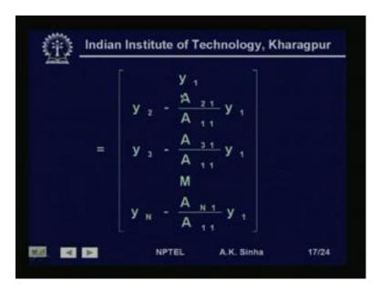
So, we can write this, when we are doing this. Of course, we are also multiplying and doing the same subtraction for the y also. So, we have y 2 is equal to A 21 by A 11 into y 1, y 3 will be equal to y 3 minus A 31 into A 11 into y 1 and so on up to y N minus A N 1 by A 11 into y 1. So, the column vector y of the known variables is also getting modified in the same way.
