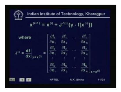
So, the iterative solution, this for iterative solution this equation, becomes likes this. X for i plus 1th iteration is equal to the value of X for i plus 1th iteration is equal to the value of X at ith iteration plus J inverse. Where we are writing d f by d x inverse as J inverse, so d f by d x is our J. So, this is J inverse at ith iteration into Y minus f X at ith iteration.
