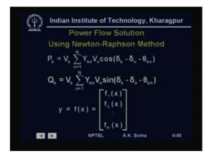
Well, as we had seen in the last lesson, the power flow equations. In terms of real and reactive power injections at any bus k is given by these relationships. So, which is a
