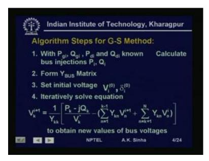
Well, as we discussed in the last lesson. The algorithm steps for Gauss Siedel method are first, what we need to do is, to find the bus injections P i and Q i. P i and Q i from the
