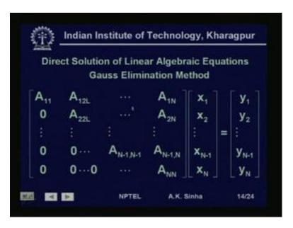
Now, how do we solve this set of equations? That is this A x is equal to y, how do we solve this kind of a system of equations. Now, what we need to do this is, if we can one method as we said earlier is take the inverse of A pre multiply it on both sides. Then, X is equal to A inverse y, that is the easiest way to do it. But, finding inverse is computationally much more complex and time consuming.
