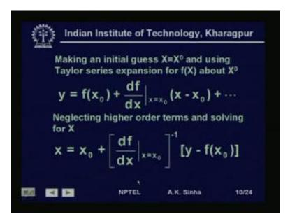
Now, if we make an initial guess X is equal to X 0. And then use the Taylor series expansion for f X about this initial guess of the state X. Then, we can write y is equal to f X 0 plus d f by d x at x is equal to x 0 into X minus X 0 plus higher order terms will be there. That is, d 2 f by d x 2, factorial 1 by 2, X minus X 0 square, all those terms higher order terms will be there.
