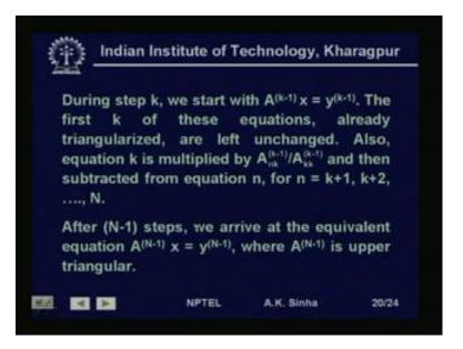
So, we can write this process as such during step k, we start with A k minus 1 X is equal to y k minus 1. This is k minus 1 is the already affected elements, that we have done at k minus 1th step. So, A k minus 1 X is equal to y k minus 1. The first k of these equations already triangularized is left unchanged, as we have seen here, if we have already triangularized this row.
