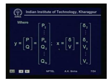
So, y is equal to f x is the general form of this equation. Now, where we have y equal to P and Q, vector P and Q are basically from P 2 to P N, P 2, P 3 upto P N and Q will be from Q 2 to Q N. That is Q 2, Q 3, Q 4 upto Q N. Now, here, what we have done is, we have assumed that bus 1, is a swing bus of slat bus. That is, for this bus, we have specified the voltage magnitude, as well x angle, the this is a reference bus.
