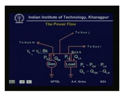
Now, if we see any busbar in detail, like if we say this busbar 2 which we have put here. This busbar, if we want to see it in detail. Then we can see this as a generator is connected to this busbar which is injecting a power real power P G K; and reactive power Q G K into this busbar. And it has load which is drawing real power P L K from the busbar and reactive power Q L K from the busbar.
