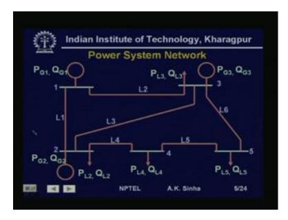
When you see this diagram, it is showing a very small power network, where we have considered 5 busbars. These busbars are can be considered in actual system as substations. So, we have say a substation which we are calling here as busbars in power system terminology, we call them as a buses. So, this bus 1 is having a generator connected to it which is supplying say real power P G 1 and reactive power Q G 1.
