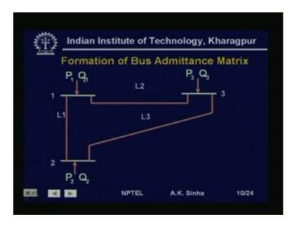
Now, let us formulate the model for this power flow analysis. In formulating the mathematical model, we need to formulate first what we call as bus admittance matrix, we will see what this actually is. Now, I have taken here a small power system with three busbars. The busbar 1 is having a real power injection P 1 and a reactive power injection Q 1, whereas busbar 2 has a real power injection P 2, reactive power injection Q 2.
