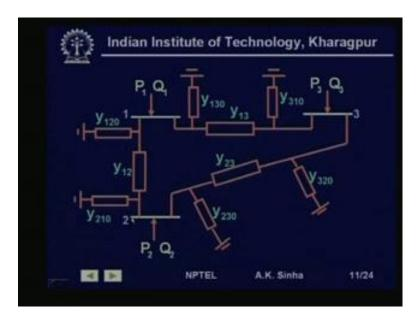
As shown here, where for a line L 1 which connecting bus 1 to bus 2, y 1 2 is representing the series admittance of the line y 1 2 0. Is representing the shunt admittance of the line, which is basically the line charging capacitance of the line and at the end towards bus 1. Similarly, y 2 1 0 is the shunt admittance of the line at the bus end 2. So, this pi equivalent model is representing line L 1 which is connecting bus 1 and 2.
