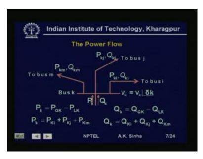
So, this can be shown as in this diagram, that is we have now instead of writing generation and loads at the busbar. We are now talking about injection into the busbar. So, if we have say load bus, then there is no generation at that bus. So, what is going to be the injection, the injection at that bus is going to be, say for that bus P k if we look at that. Then, we have no generation that is P G K is 0, then P k is equal to minus P L K and similarly, Q k will be equal to minus Q L K.
