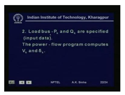
Then, other type of busbar is a load busbar, where both real and reactive powers are specified. In at this busbar what are the unknowns, if we know V and delta at this busbar, we have all the variables. So, here P and Q are specified, that is injection real and reactive power injection is specified. And the unknowns at this busbar are V and delta a voltage magnitude and it is phase angle.
