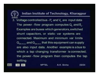
We have a third type of busbar, which we called as voltage controlled busbars. These are generally busbars, where we have generation at these busbars P k and V k are specified. That is the real power and the voltage magnitude is specified and the power flow
